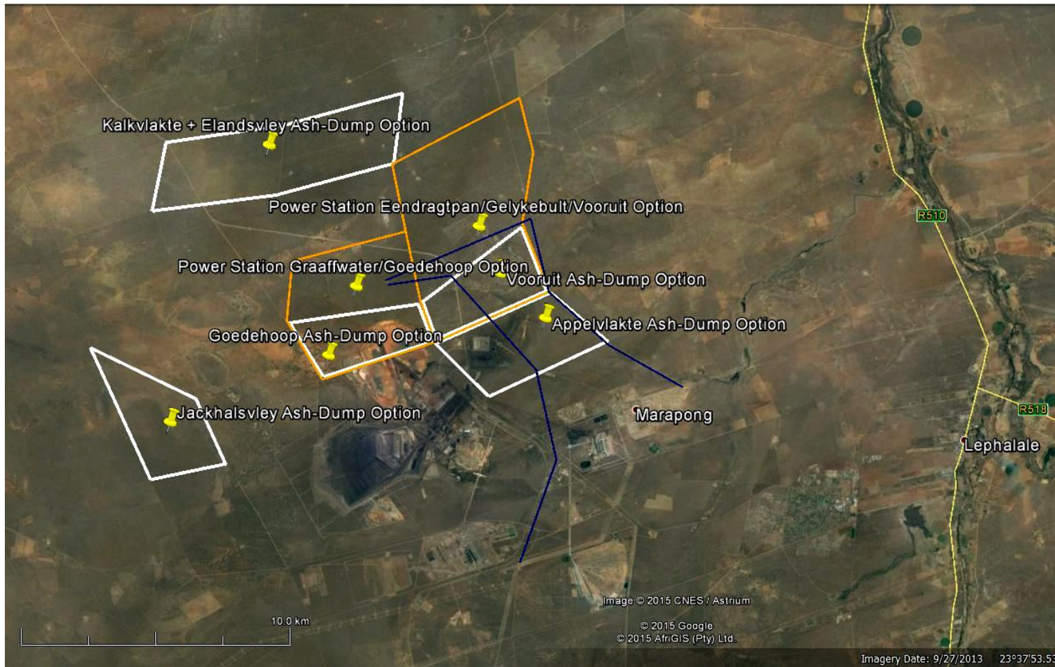
Figure 2. Google earth© satellite image of the Tshivhaso Coal-fired Power Plant study area c. 20 km to the NW of Lephalale, Limpopo (land parcels outlined in white) to the north of the existing Grootegeluk opencast mine. Land parcels under consideration for the power plant are outlined in orange; those being considered for the ash-dump are shown in white. Grid connection options are indicated in blue.
