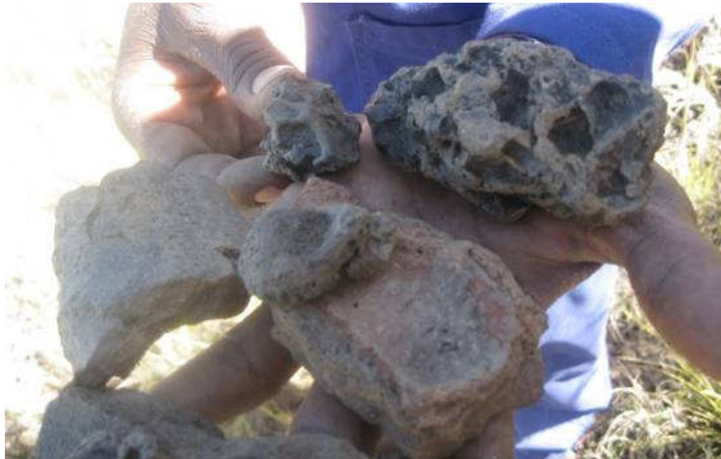
Figure 28. Slag and pieces of tuyere from the smelting site.
