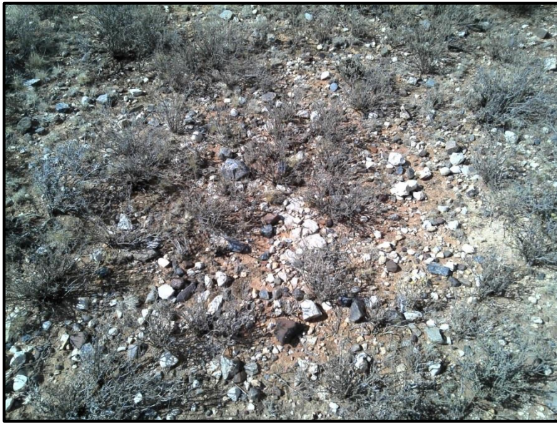
Figure 2. Calcrete and gravel that is found in large portions of PV West
