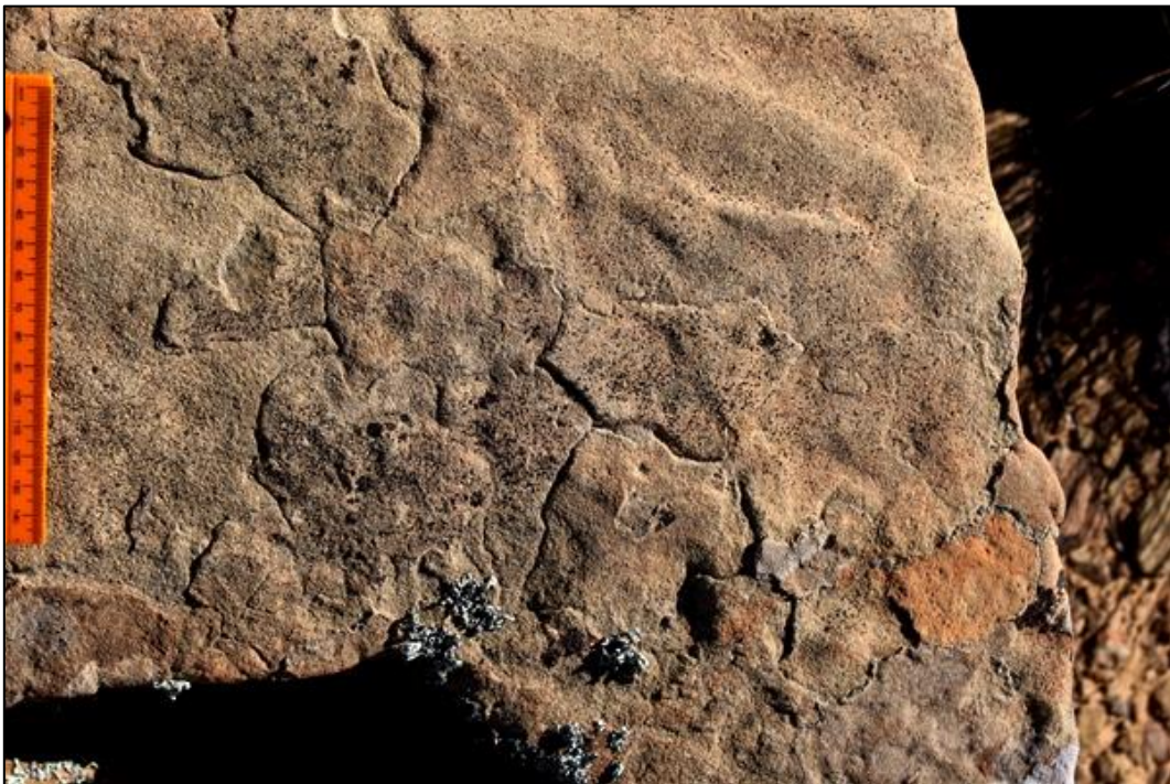
Figure 13: Typical patchwork of irregular, superficial depressions and ridges generated by biological weathering of sandstone by lichens (Scale in cm and mm).
