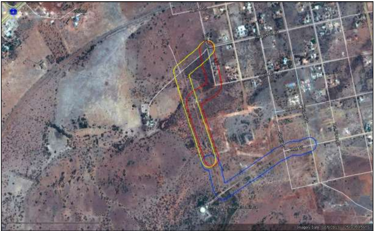
Figure 2. Google earth© satellite image of the study area on the south-western outskirts of Zeerust showing 50 m-wide corridors for the three access route options to the approved solar energy facility: Alternative 1 (preferred, yellow), Alternative 2 (red), Alternative 3 (blue). Note the highly disturbed terrain and low level of bedrock exposure here.
