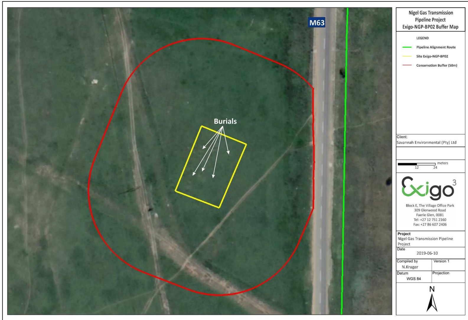
Figure 6-2: Aerial image indicating the 50m conservation buffer required for Site Exigo-NGP-BP02 in relation to the proposed pipeline alignment (green line).
