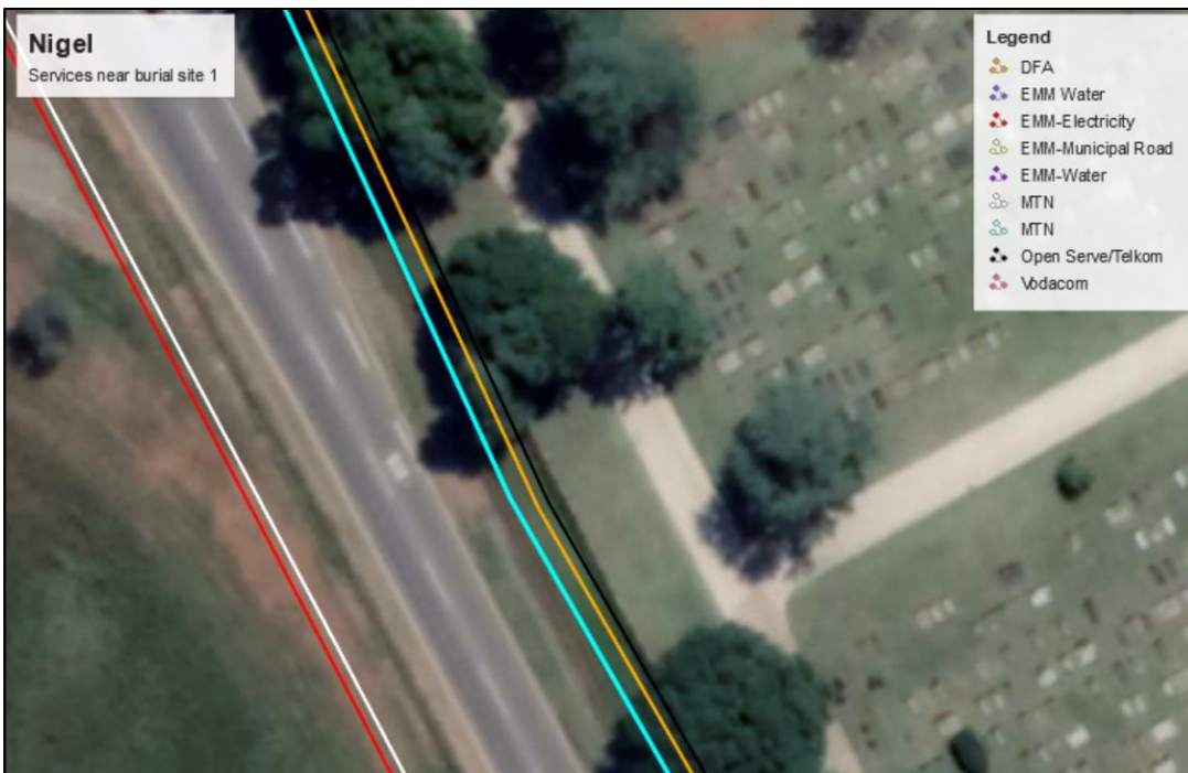
Figure 5-6: Google Earth image of existing municipal services present in the servitude of the M63 road in the vicinity of the municipal cemetery at Site Exigo-NGP-BP01 (image provided by client).
