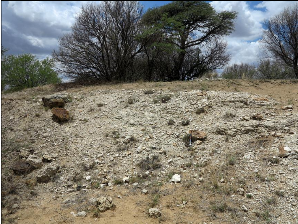
Fig. 9. Cut face in the borrow pit illustrated above excavated showing thick calcretised pan deposits with dispersed boulder-sized blocks of Boomplaas Formation bedrocks (Hammer = 30 cm).
