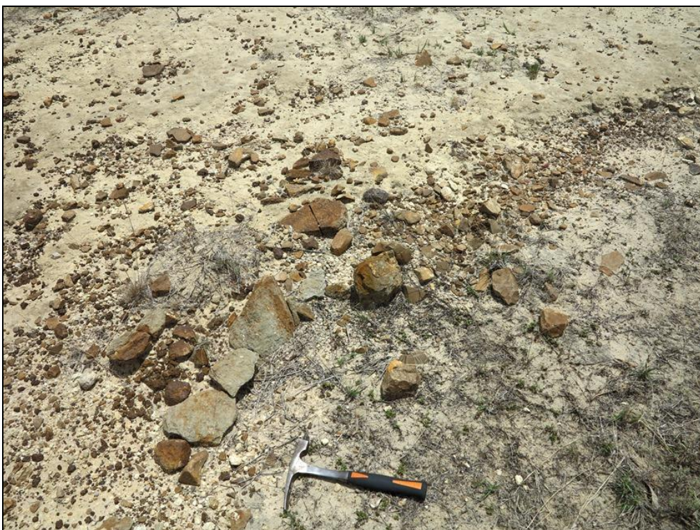
Fig. 10. Horizon of angular quartzitic gravels within the calcretised pan sediment succession (Hammer = 30 cm).
