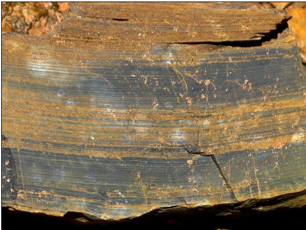
Fig. 24. Close-up of finely-laminated dark grey mudrocks from the Boomplaas Formation (Block is 6 cm thick).
