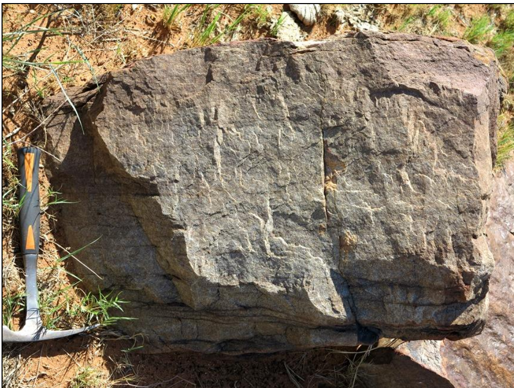
Fig. 9. Block of tough, greyish Vryburg Formation quartzite showing faint cross-lamination and occasional dark heavy mineral laminations or flasers (Hammer = 30 cm).
