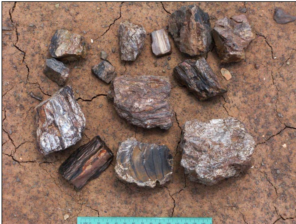
Fig. 31. Assortment of cherty clasts of petrified wood from surface gravels at Loc. 034 (Scale in cm and mm). Note lack of rounding suggesting limited transport.
