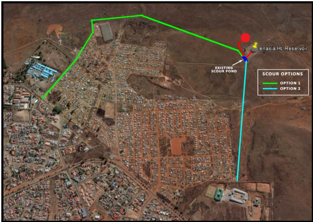
Figure 8: Options to drain scour pond
