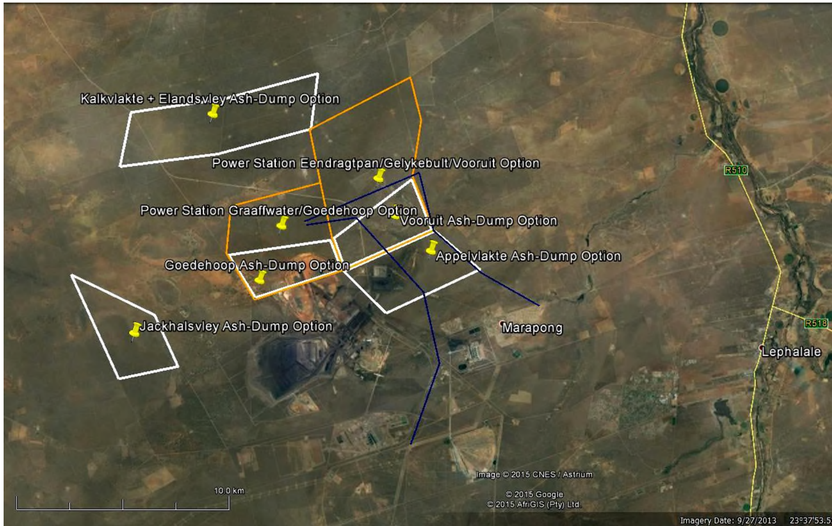
Figure 2. Google earth© satellite image of the Tshivhaso Coal-fired Power Plant study area c. 20 km to the NW of Lephalale, Limpopo (land parcels outlined in white) to the north of the existing Grootegeeluk opencast mine. Land parcels under consideration for the power plant are outlined in orange; those being considered for the ash-dump are shown in white. Grid connection options are indicated in blue.
