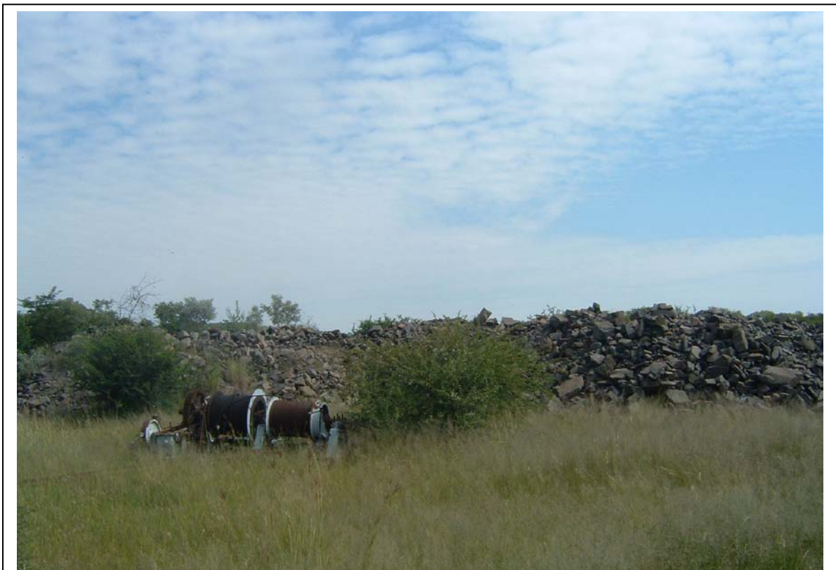
Figures 10 & 11- The anchor concrete block on which the mine's head gear rested (below), this is the most pronounced feature to be associated with the chrome mine (above). Pulleys with cables hoisted coco pans from the underground mine to the surface where the chrome ore was stock-piled (above).
