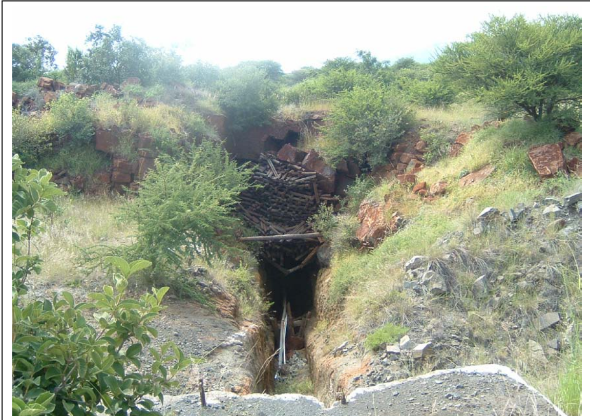
Figure 9- An incline shaft running into the chrome mine on Witkleifontein 136JP and Rooderand 46JQ. Note the corridor with a railway line between the shaft and the anchor block.
