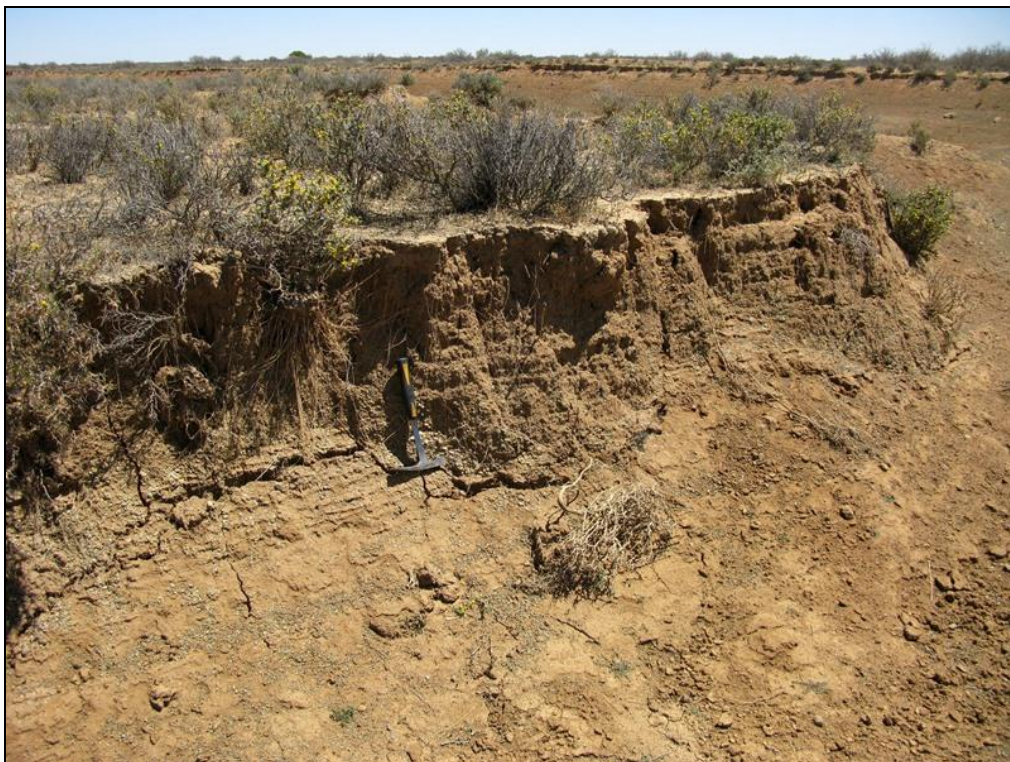
Fig. 23. Borrow pit section through thinly-bedded silty sediments overlying Dwyka bedrocks, perhaps related to a pan area, Farm 246 (Hammer = 30 cm).
