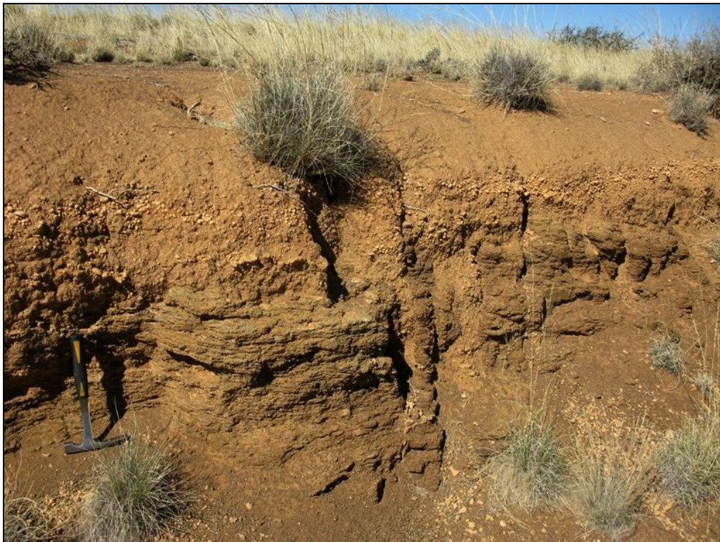
Fig. 33a. Deeply-weathered dolerite sabunga overlain by silty alluvial soils with nodular calcrete horizon, borrow pit on Kopjes Vlei 281 (Loc. 040) (Hammer = 30 cm).
