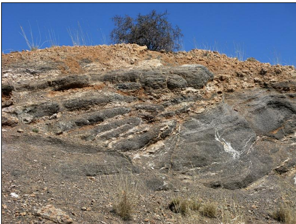
Fig. 33b. Extensive calcrete veining of deeply-weathered dolerite sabunga exposed in a borrow pit on Olyven Kolk 187 (Loc. 050).
