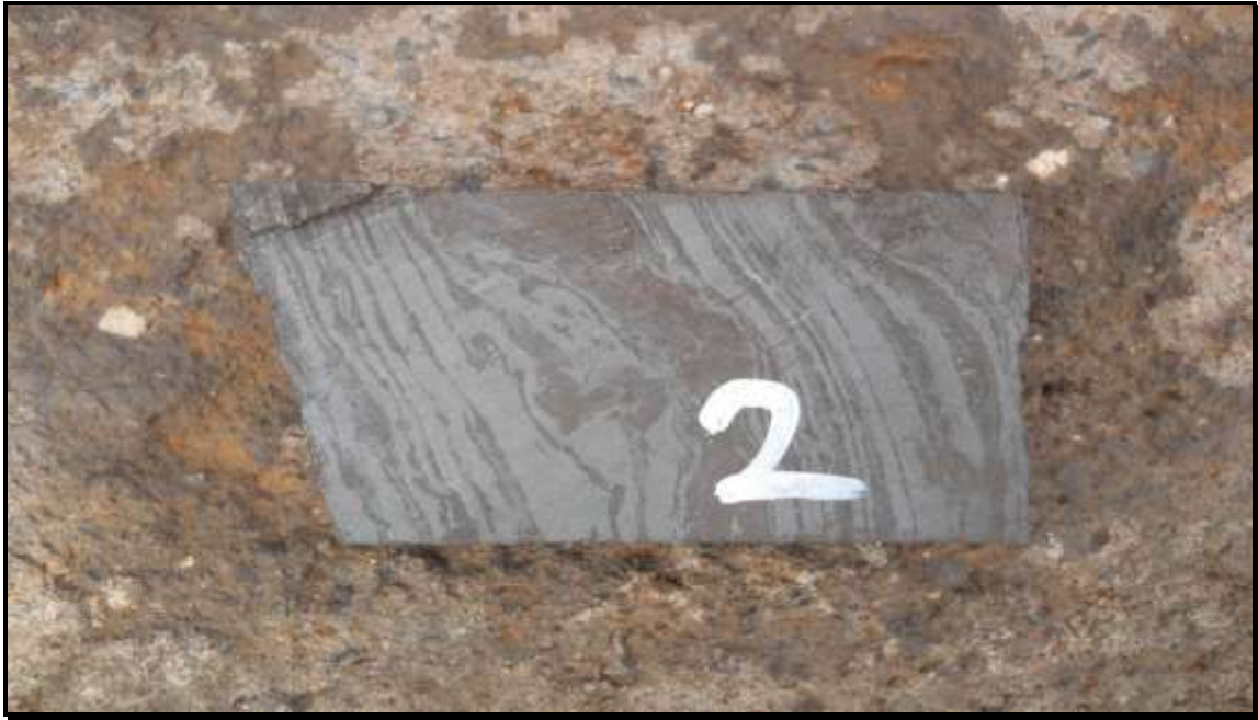
Figure 4.6 Algal structures associated with banded iron units in the Hotazel Formation, as seen in some of the borehole logs in the study area.
