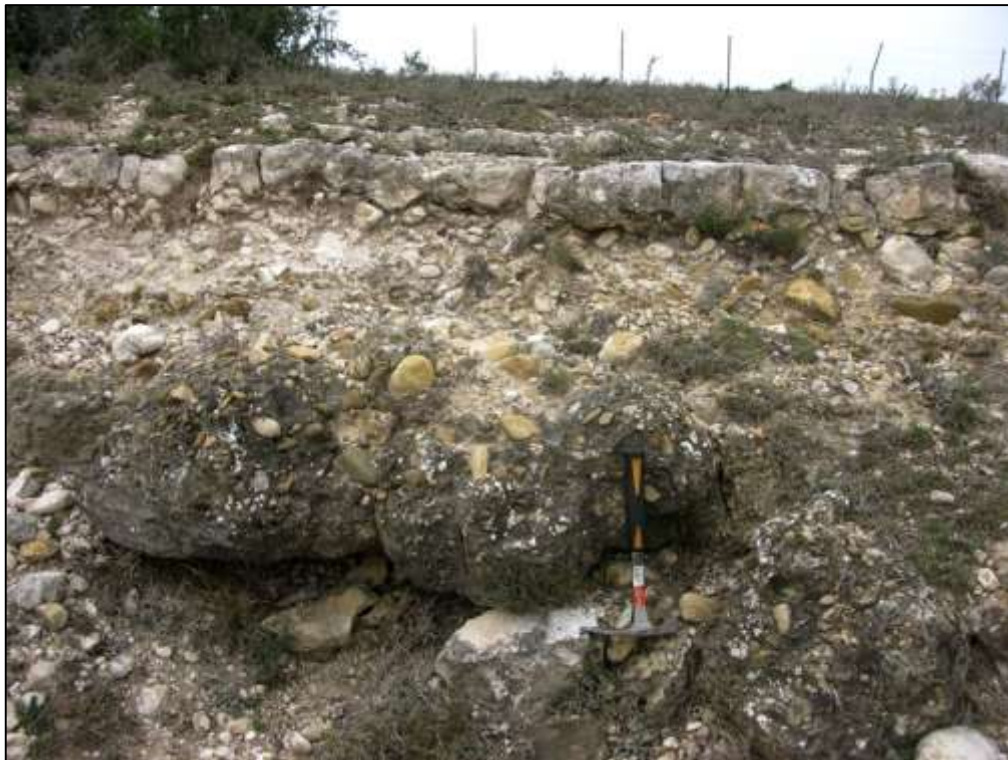
Fig. 47. Conglomeratic basal beds of the Alexandria Formation capped by calcretised calcarenites, Gringley 188 (Loc. 689) (Hammer = 30 cm).
