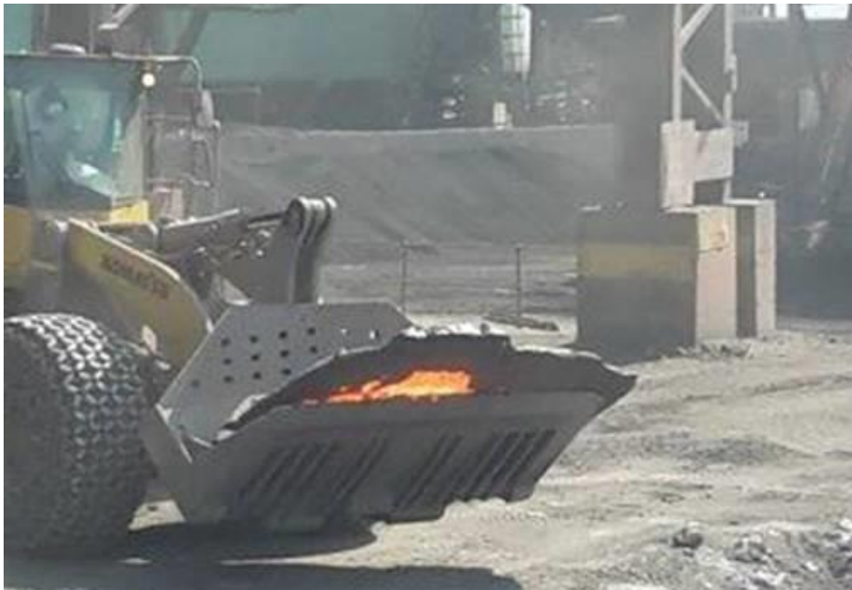
Figure 6: Chrome Slag being removed from the smelting process.
