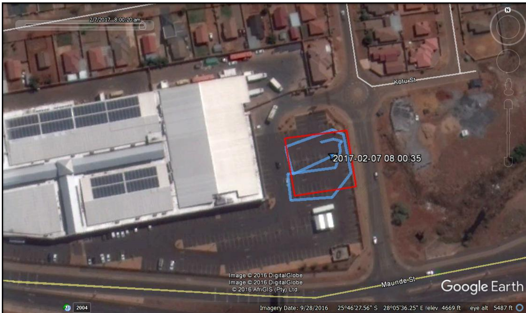
Figure 3. Track logs of the areas surveyed indicated in blue with the development footprint indicated in red.
