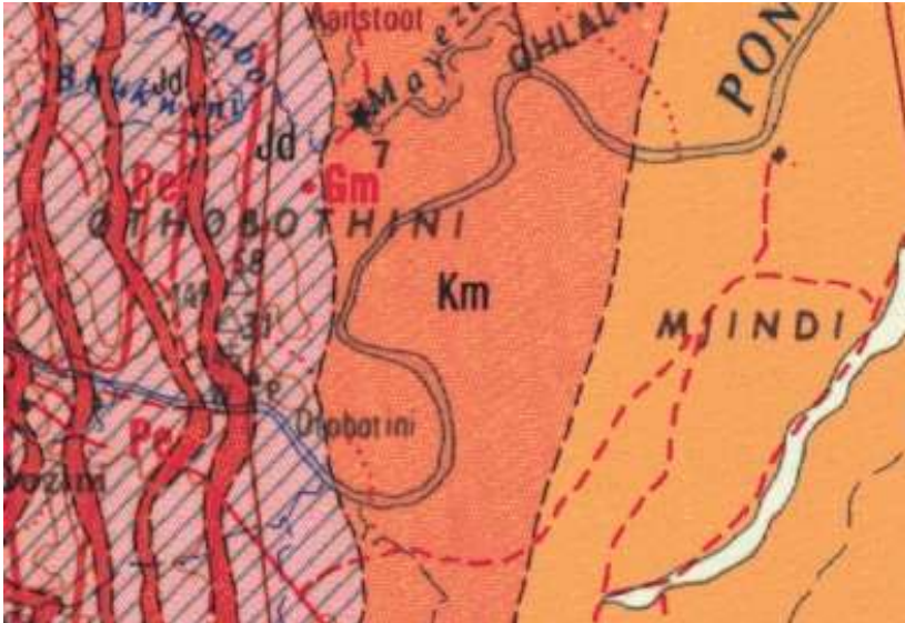
Figure 2: Extract from the Kosi Bay 2632: 250 000 scale Geological Map showing the area of interest. The proposed Makatini Pedestrian Bridge will be located on the Makatini Formation (Km).
