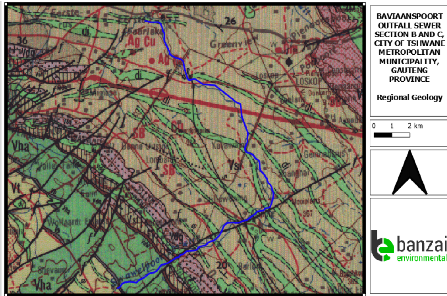
Figure 4: Extract of the 1:250 000 2528 Pretoria Geological map (Council of Geoscience) of the proposed Baviaanspoort Outfall Sewer (Section B and C), Tshwane Metropolitan Municipality, Gauteng Province (development footprint indicated in yellow). Map drawn by QGIS 2.18.28.
