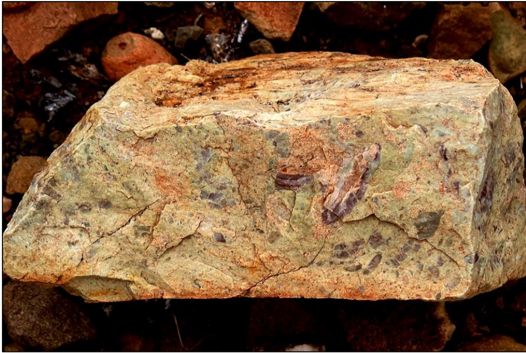
Figure 40: Block (c. 12 cm long) of quartzose mylonitic crush breccia associated with low angle thrust faults such as that illustrated above.
