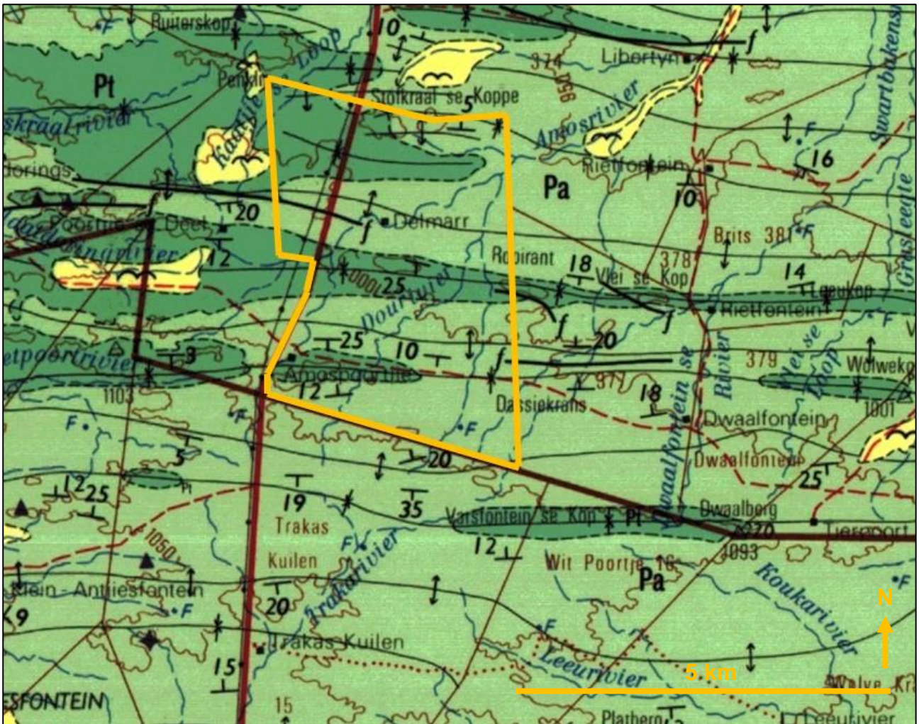
Figure 10: Extract from 1: 250 000 geology sheet 3222 Beaufort West showing the boundaries of the Kraaltjies WEF project area to the south of Beaufort West (orange polygon). Note numerous W-E trending fold axes occur in the region which falls within the northern margins of the Cape Fold Belt. Pa (pale green) = Abrahamskraal Formation (Adelaide Subgroup, Lower Beaufort Group). Pt (dark green) = Poortjie Member of the Teekloof Formation (Adelaide Subgroup, Lower Beaufort Group). Yellow = Late Caenozoic / Quaternary superficial sediments, including alluvium (flying bird symbol), as well as unmapped sheet wash, colluvium, soils, locally cemented by pedocretes such as calcrete. To the west of the N12 and outside the WEF and associated Infrastructure project area diamond symbols indicate fossil localities within the Tapinocephalus Assemblage Zone. Triangles indicate fossils within the Pristerognathus Assemblage Zone (N.B. This fossil biozone data is now outdated and the fossils concerned have probably been collected).
