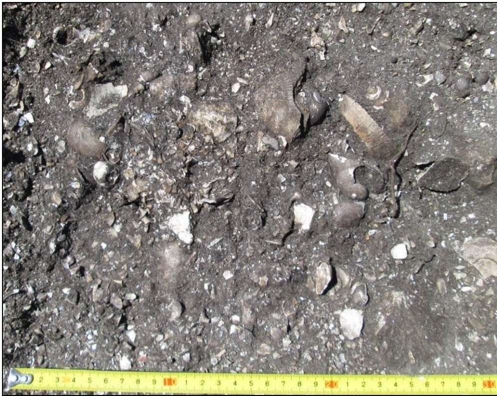
Figure 12: Close-up photograph of the CFS deposits showing the finely fragmented and highly compacted shell.
