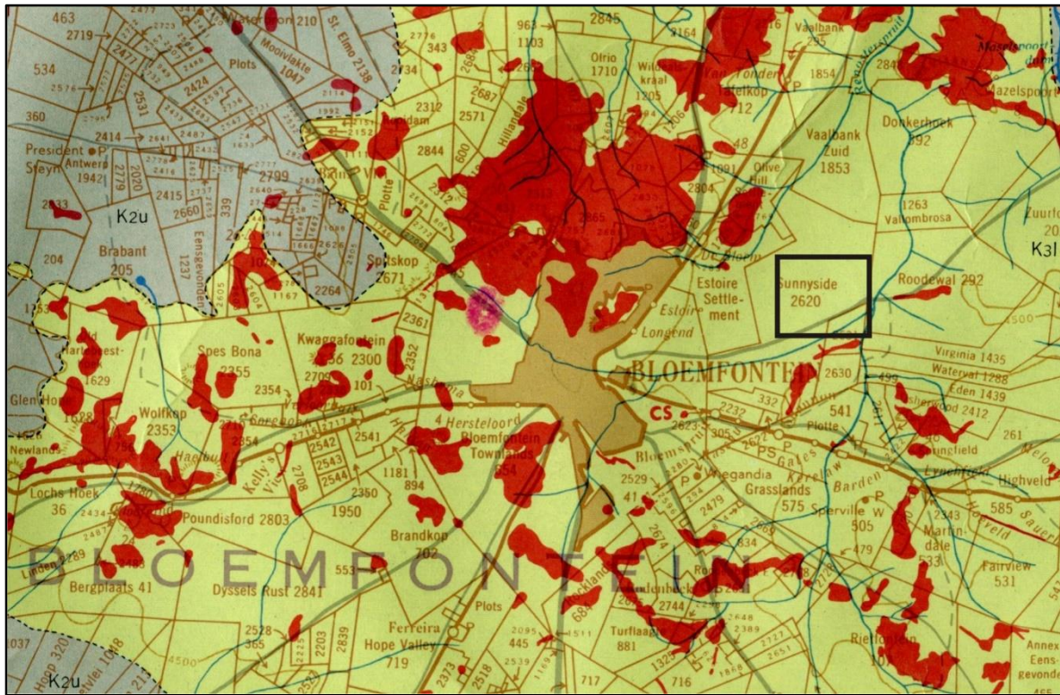
Figure 5. The surface geology of the proposed township development in Bloemfontein, indicated by a black square. Note that the position of the roads in the area has not been updated. The development area is underlain by Late Permian, Dicynodon Assemblage Zone. (Modified from the 1: 250 000 geological map 2926 Bloemfontein (Council for Geoscience, Pretoria).
