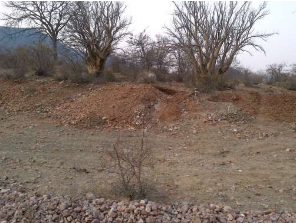
Figure 7: View of the Geotech test pits on borrow pit 03.
