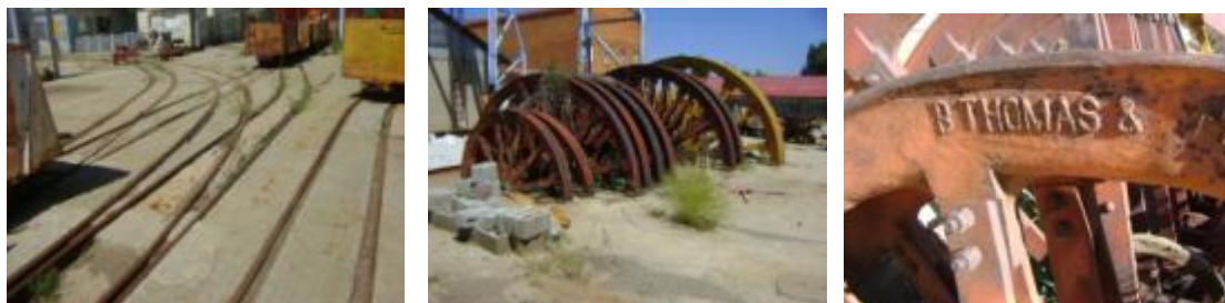
Figs. 21 to 23. Above are typical rails, coco-pans, rope wheels and structures on site of #1 shaft. All of the infrastructure is to be retained, upgraded to modern safety regulations and re-used. (Photographs, S.M. Miller 2015.)
