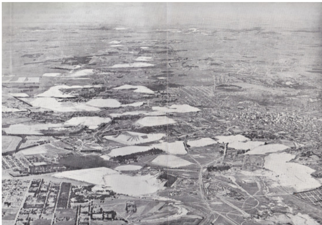
Fig. 09. Above. Looking west from above Johannesburg at City Deep mine along the Main Reef. In the background can be seen the Krugersdorp/Randfontein mines. The large break between mine dumps is indicative of the Witpoortjie fault-line. This image is indicative of the position of the reef and its richness in yield. The image dates from circa 1938. ( Haughton, 1940, opposite pp-118. )
