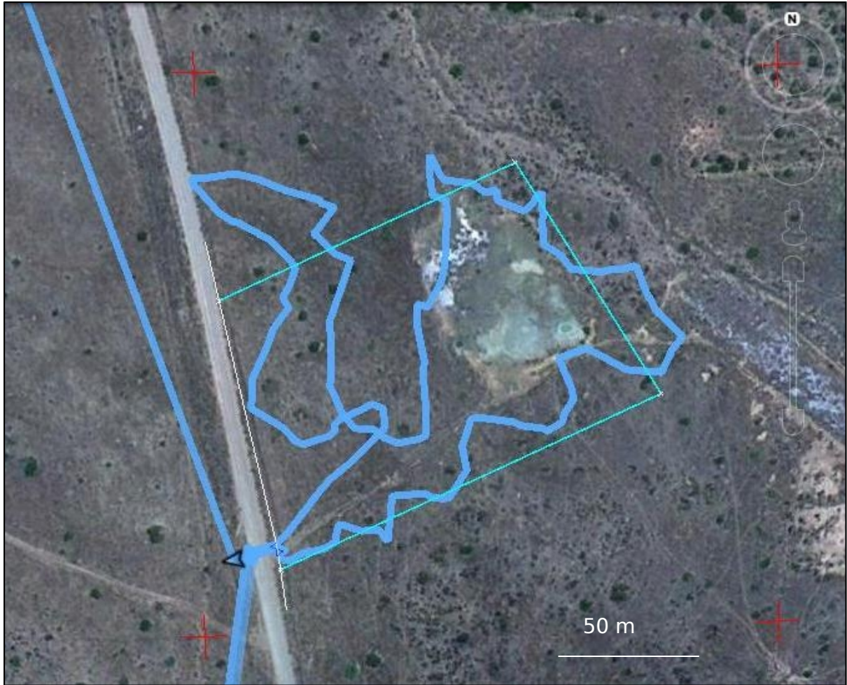
Figure 7: Google earth image showing the proposed extension of the existing borrow pit 108 and the tracks of the field survey. Please note that the straight blue lines do not indicate survey tracks.
