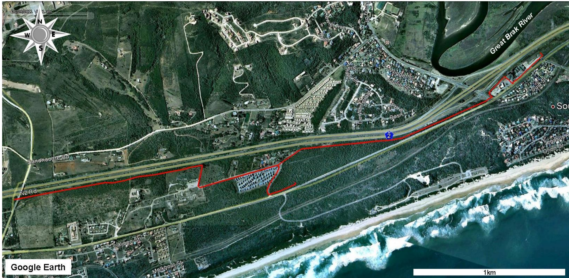
Figure 3. Enlarged area as indicated in Figure 1 showing the proposed Midbrak Main Sewer Pipeline route in red.
