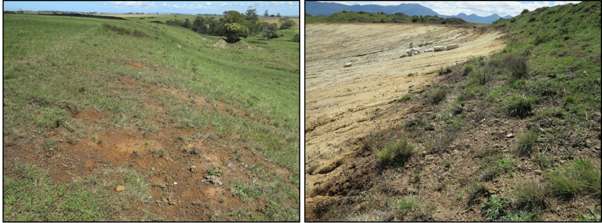
Figure 7 and 8: View towards the southwest of the slope where there is exposure of the underlying ground; view towards the northeast with the ferruginised gravel layer visible in the foreground.
