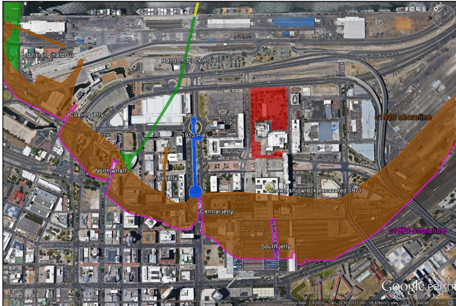
Figure 2: Table Bay harbour - historical development 1870-1985 (based on: South African Transport Services Drawing TBH 106 (1985): A-374). Proposed development site shown in red. The area between the 1920 shoreline and the existing harbour was reclaimed between 1938 and 1943. Comparison with the 1926 aerial photo in Figure 7 shows that the information with regards to the 1920 shoreline omits certain features such as the Rogge Bay fishing “harbour”.
