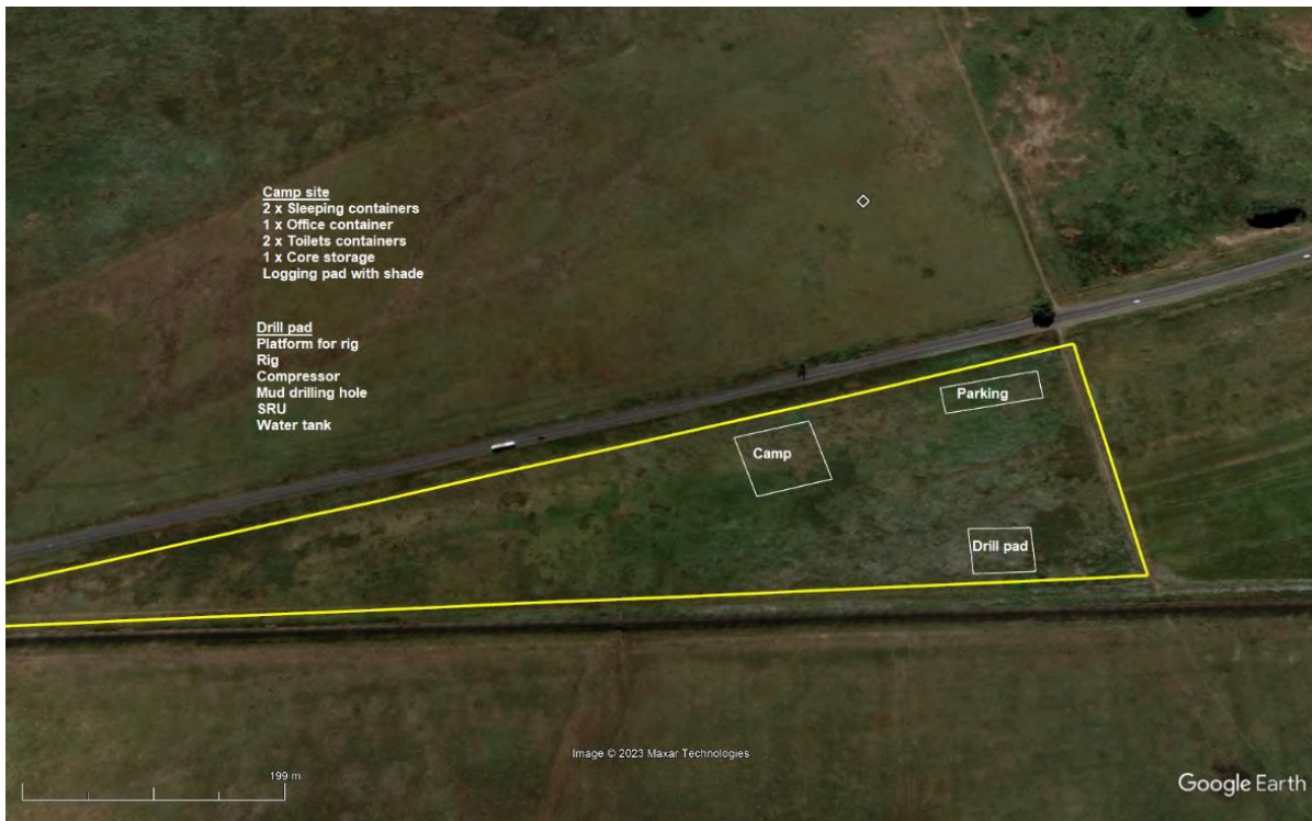
Figure 4: Schematic of proposed drill site (Nemaï, 2023)
