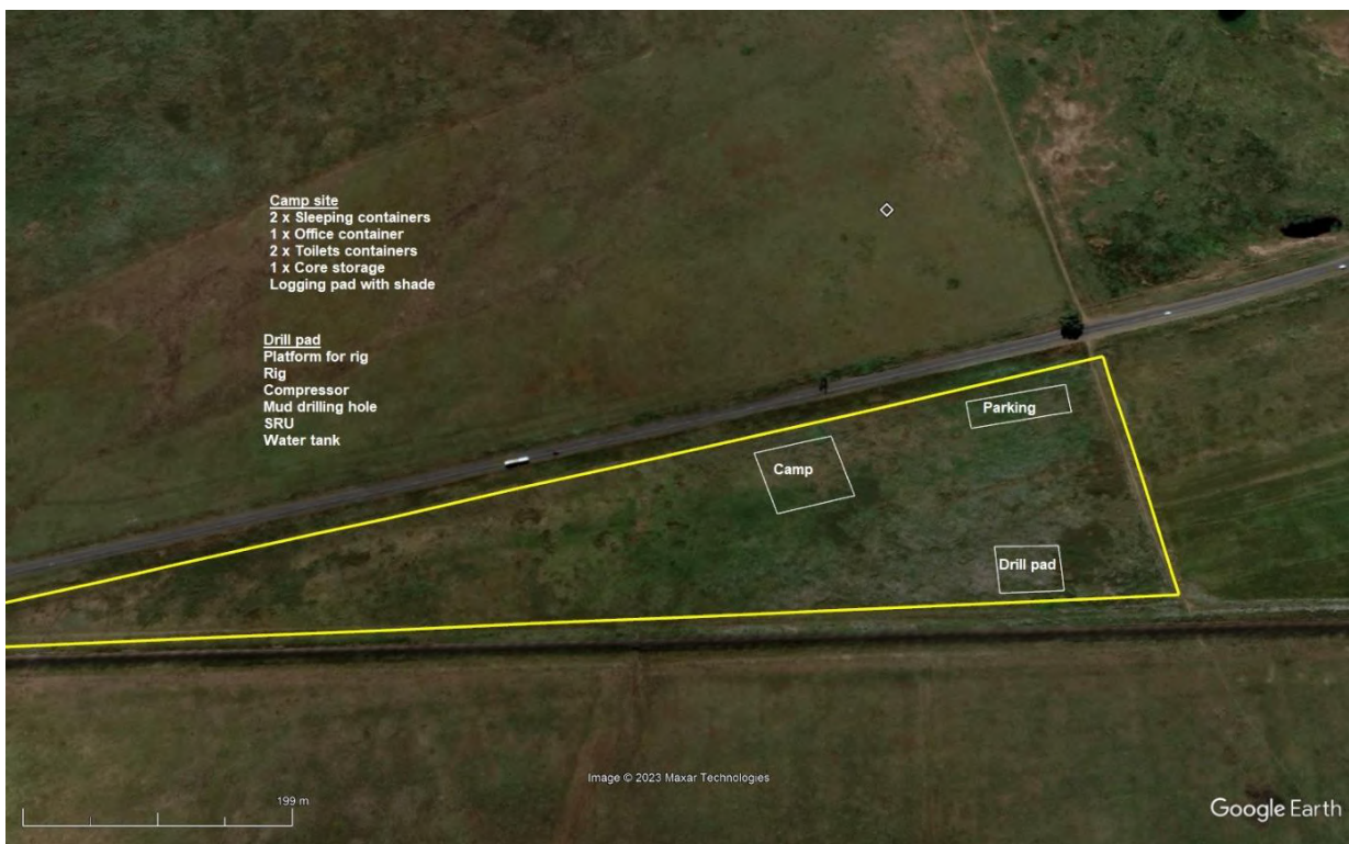
Figure 26: Proposed Drilling Site updated Schematic showing position of drill pad close to the approximate location of the possible grave CCUS-02
