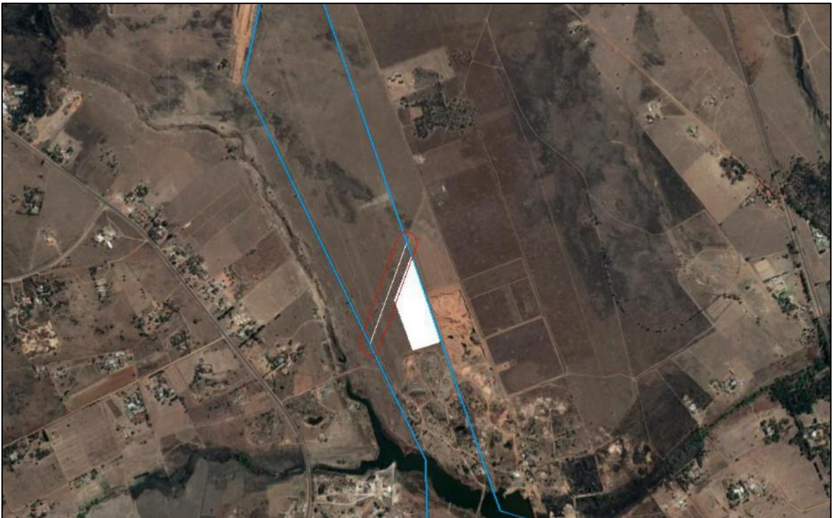
Figure 6-1: 50 m buffer delineated around SASOL pipeline to avoid risk (RED: 50m Buffer)
