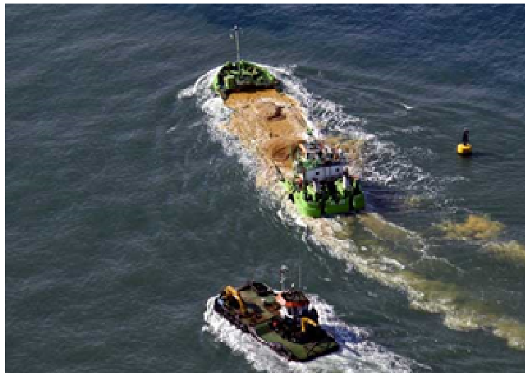
Photo 1: Dredger transporting spoil for disposal to an offshore disposal site.
