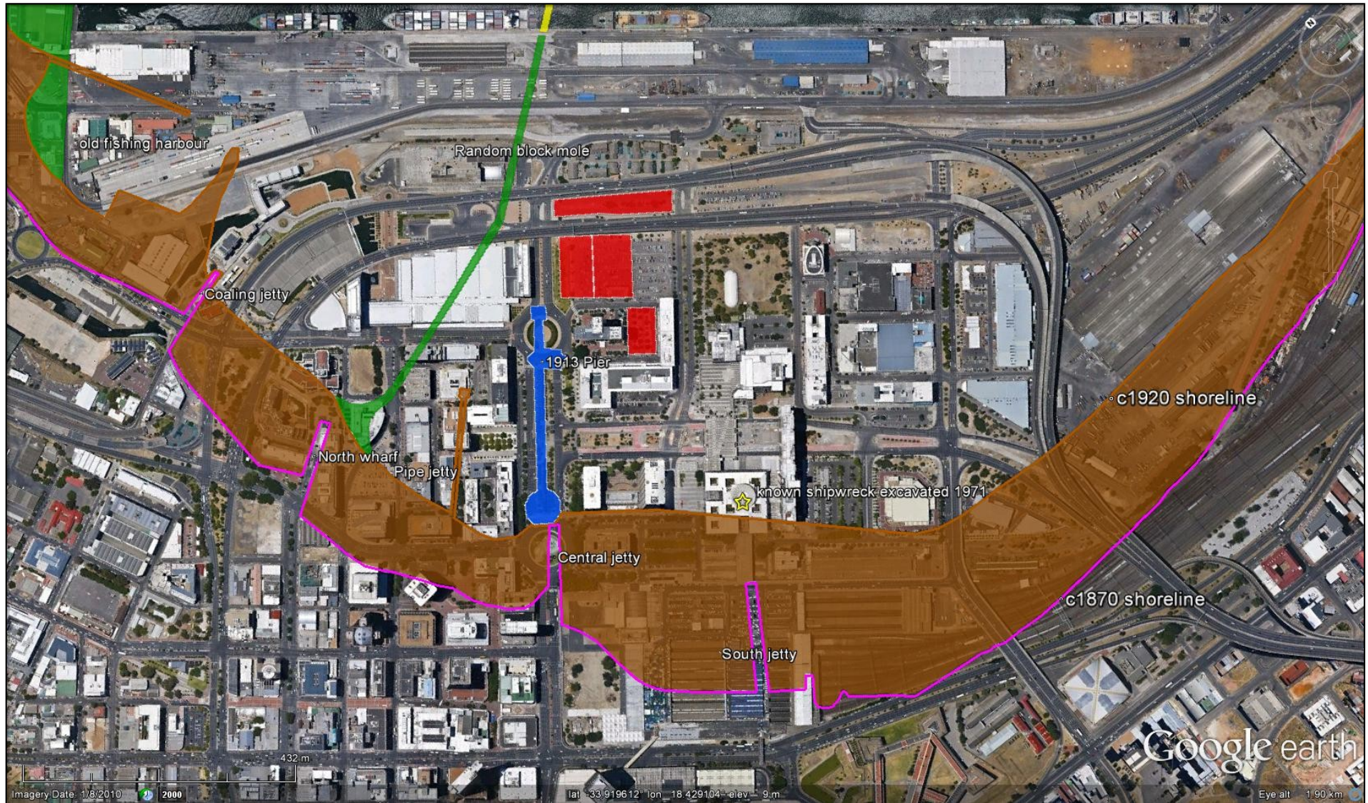
Figure 2: Table Bay harbour - historical development 1870-1985 (based on: South African Transport Services Drawing TBH 106 (1985): A-374). Proposed development sites shown in red. The area between the 1920 shoreline and the existing harbour was reclaimed between 1938 and 1943. Comparison with the 1926 aerial photo in Figure X shows that the information with regards to the 1920 shoreline omits certain features such as the Rogge Bay fishing “harbour”.
