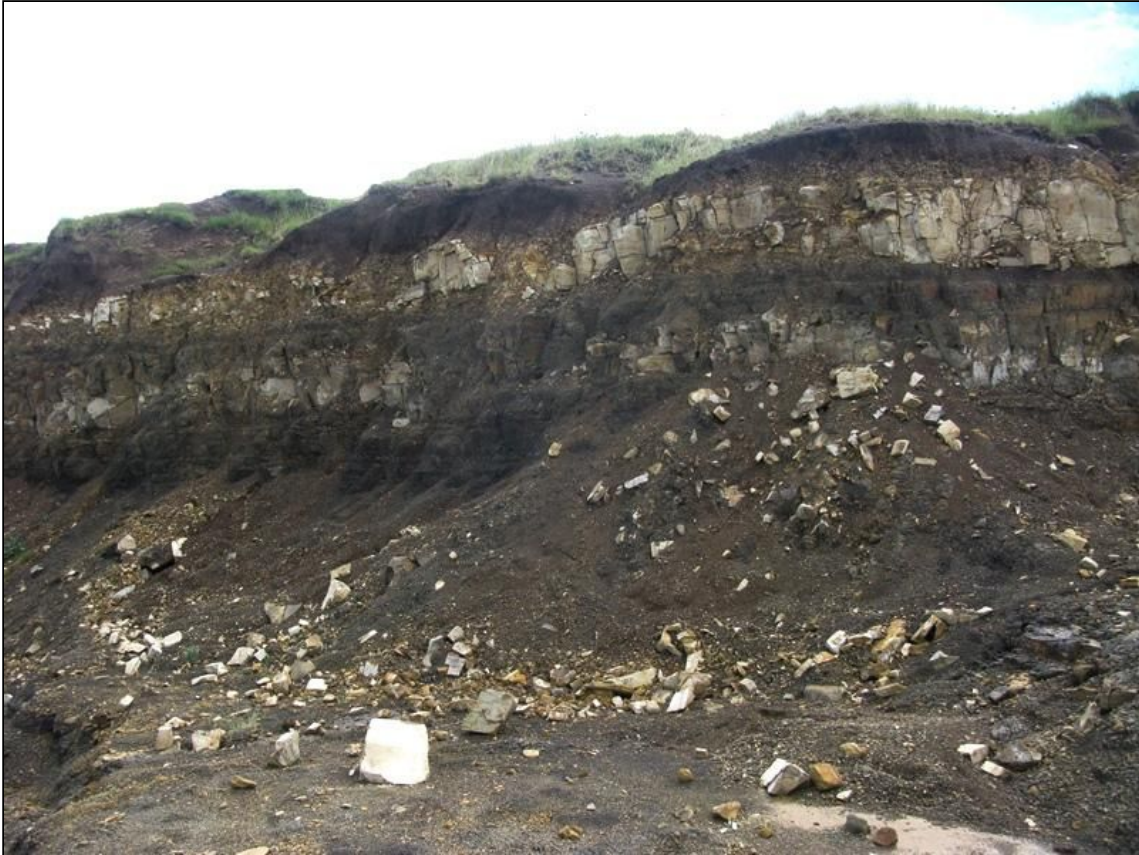
Figure 12. Borrow pit cut face exposing pale tabular-bedded sandstones and thinner-bedded, dark grey-green mudrocks of the Balfour Formation (BP16, Loc. 048).
