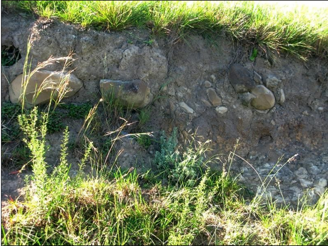
Figure 30: R63 road cutting exposing coarse, poorly-sorted, gravelly colluvial sands and grits overlying weathered Balfour Formation saprolite (Loc. 071).
