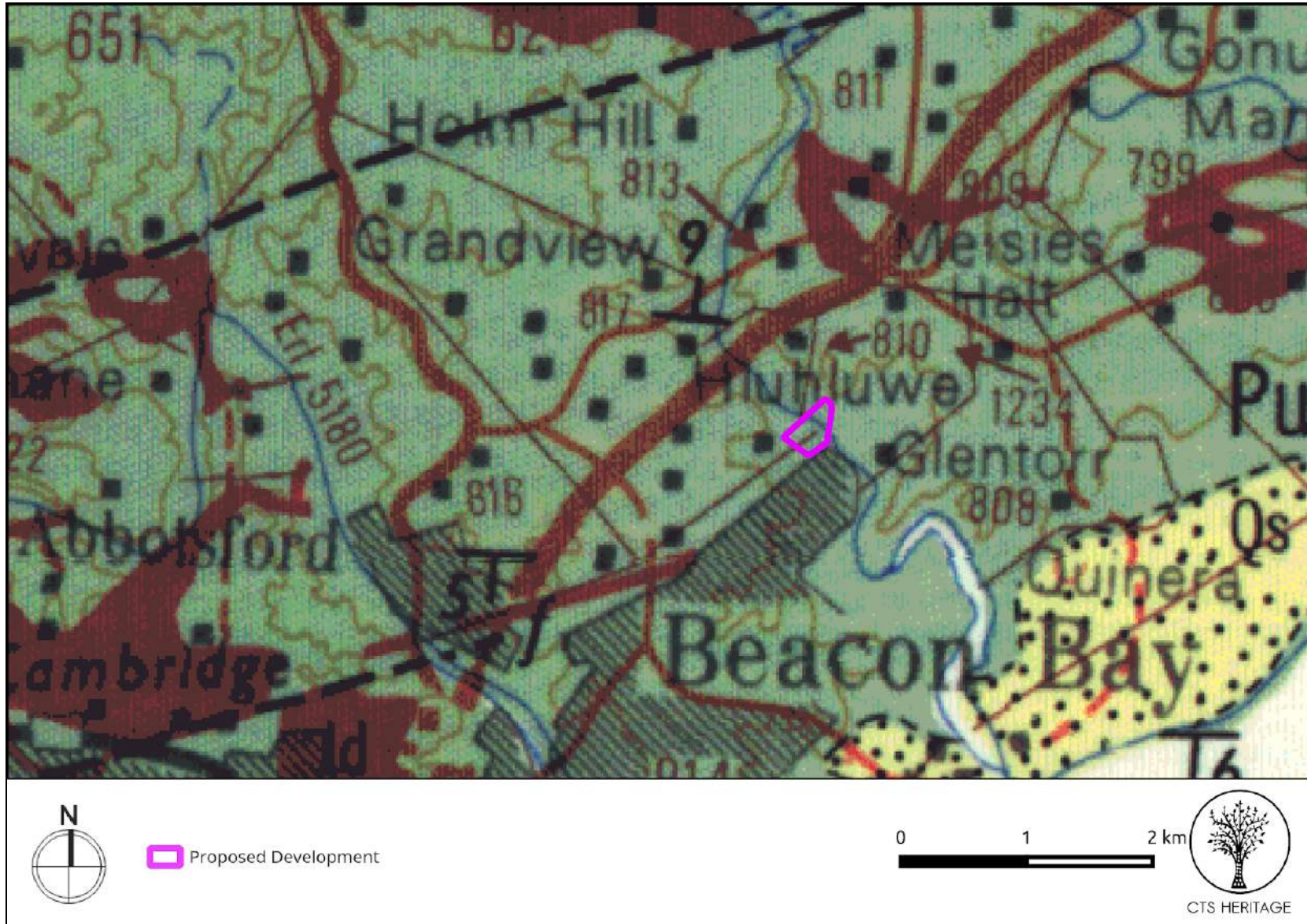
Figure 6. Geology Map. Indicating the underlying geology across the study area through overlaying the geology maps from the CGS series 3226 King Williams Town (Pub: Balfour Formation (Grey mudstone, shale, sandstone))
