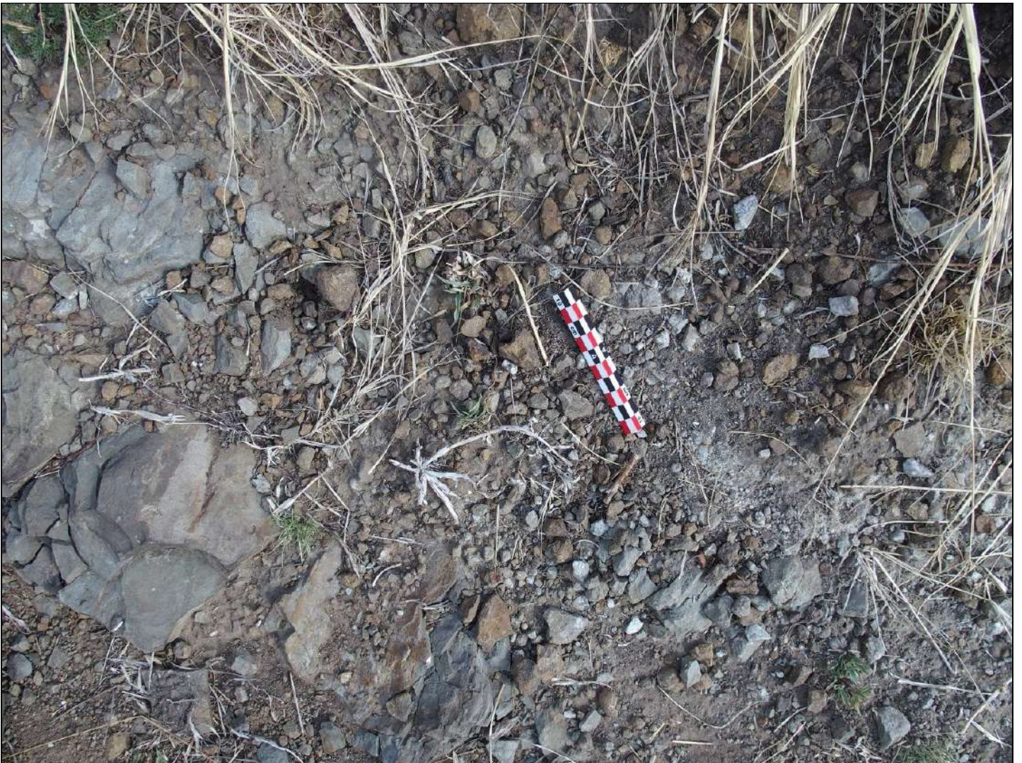
Figure 5.9: Greyish medium grained mudstone under dam outcrop probably from the Adelaide Subgroup (scale bar = 10cm)
