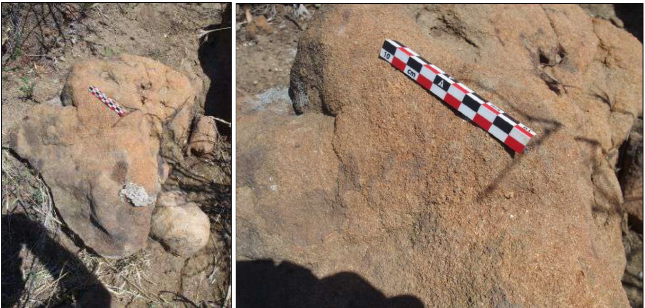
Figure 5.2: Outcrop 2 (scale bar = 10cm) consisting of medium to coarse grained yellowish sandstone (probably of the Adelaide Subgroup)
