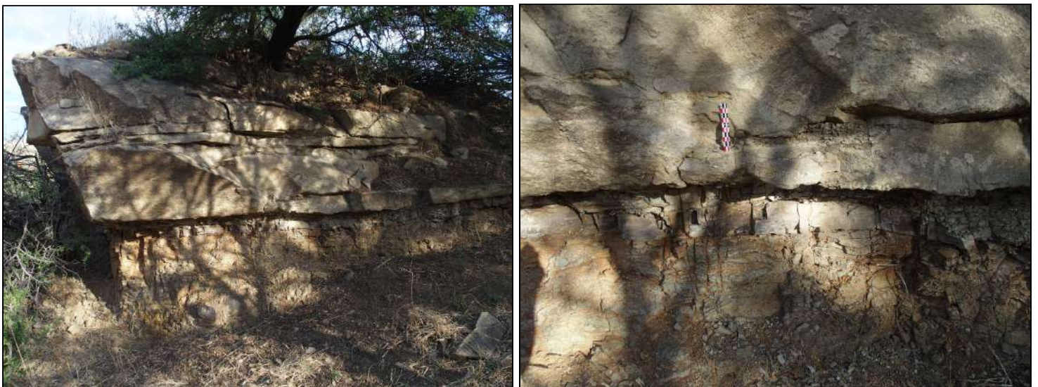
Figure 5.11: Outcrop 5 consisting of medium to coarse grained yellowish sandstone underlain by greyish to greenish medium grained mudstone (probably Adelaide Subgroup) (scale bar = 10cm)
