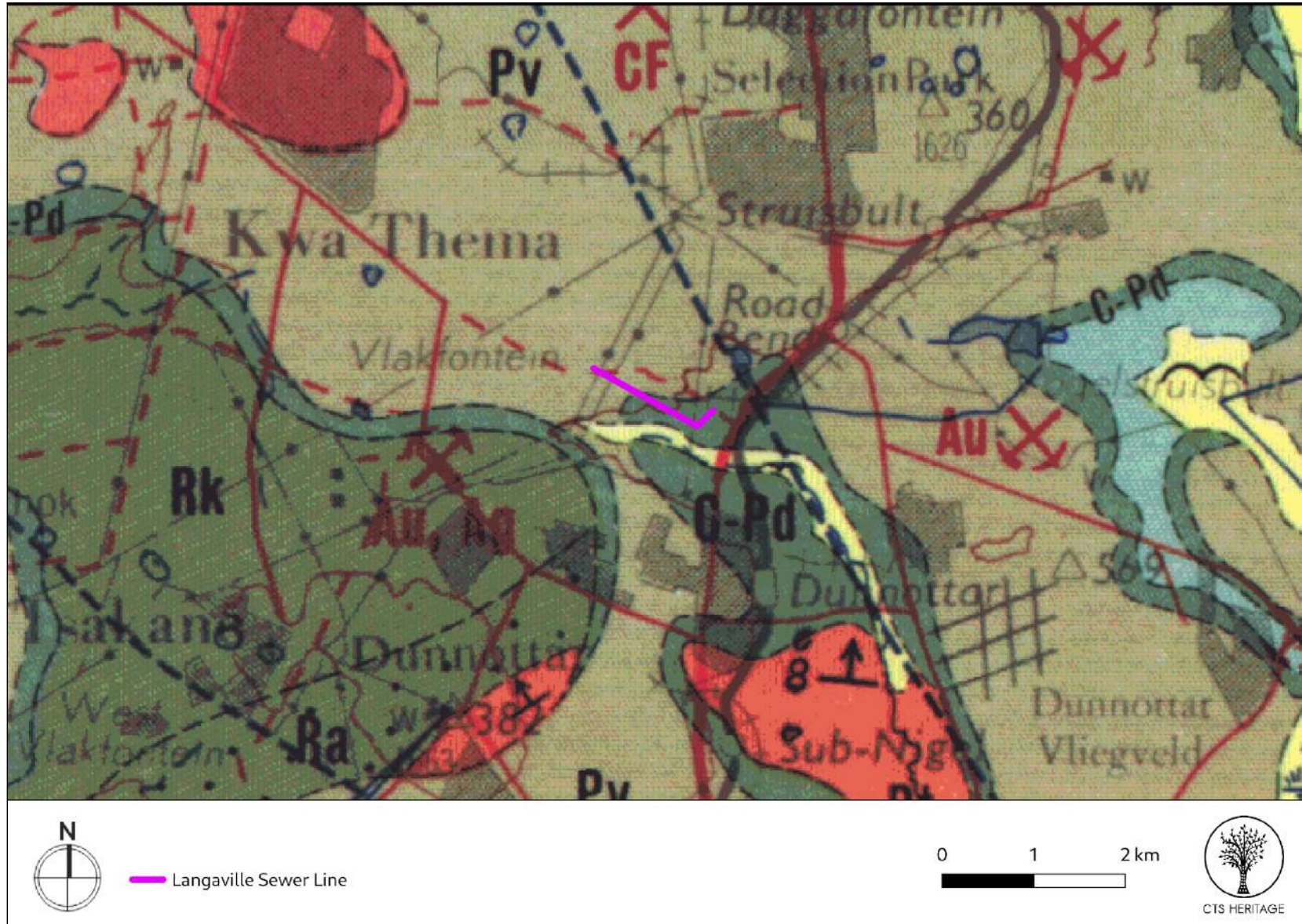
Figure 5. Geology Map. Extract from the Council for GeoScience East Rand Map 2628 indicating that the area proposed for development is underlain by Pv: Vryheid Formation and C-Pd: Dwyka Formation of the Ecca Group
