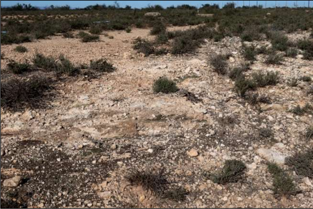
Figure 29: Pale, creamy, calcretised younger alluvium exposed in a borrow pit along the Gannaleegte on Doorn Poort 93. The underlying fractured siltstone bedrocks are also extensively veined by calcrete.
