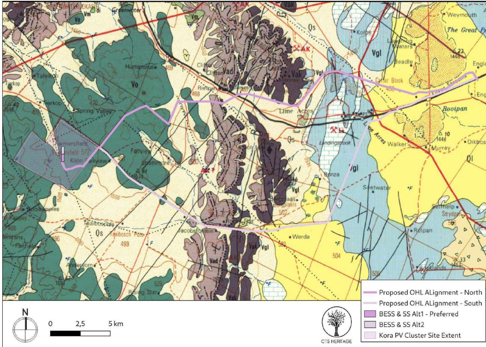
**Figure 4b. Geology Map.** Extract from the CGS 2822 Postmasburg Map indicating that the development area is underlain by sediments of the Vo: Ongeluk Formation, Vad: Danielskuil Member and Vak: Kuruman Member of the Asbesberge Formation, Vgl: Lime Acres Member of the Ghaap Plateau, Ql: Surface Limestone and Qs: Quaternary Sands
