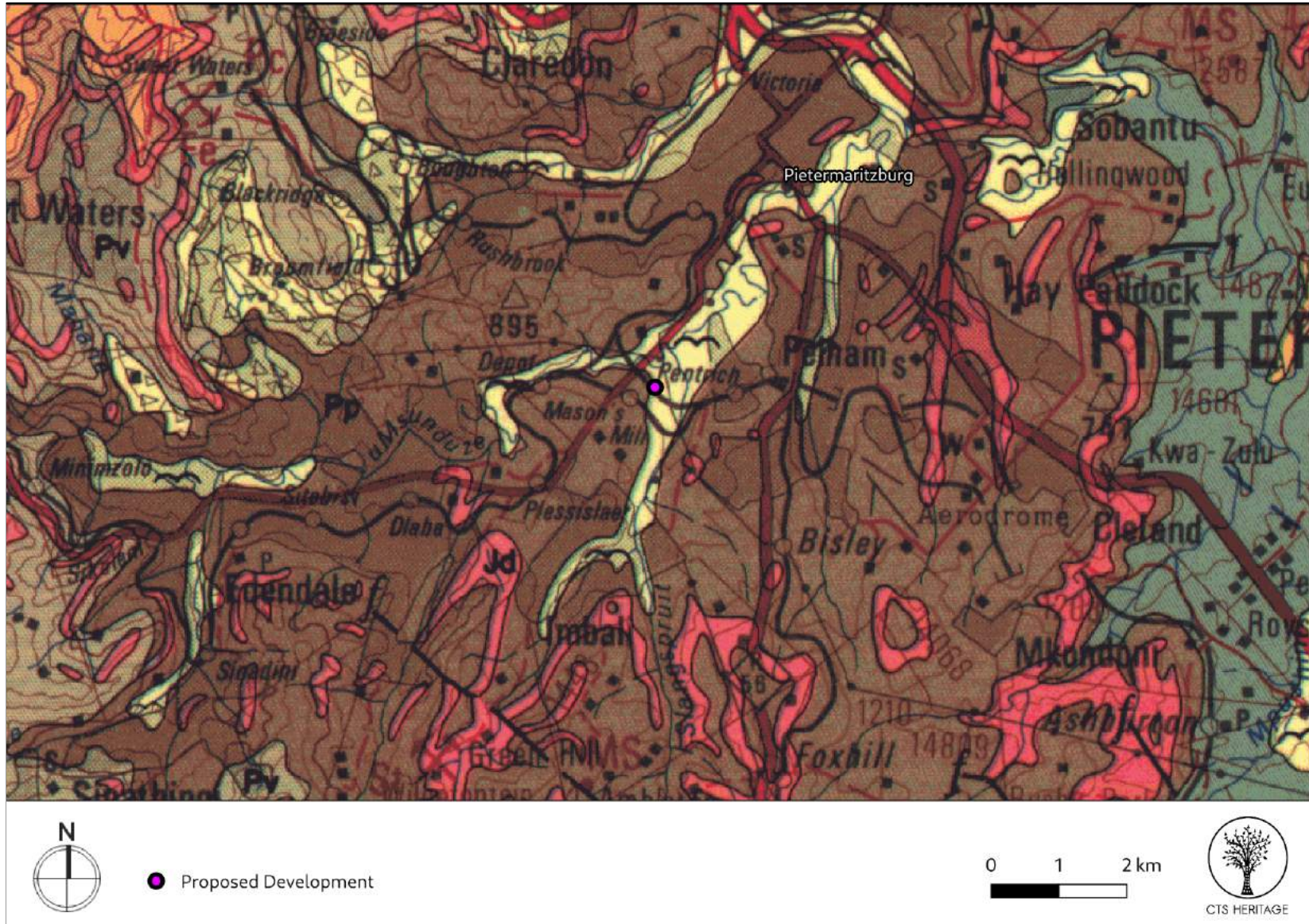
Figure 4b. Extract from the CGS Map. Extract from the Council for GeoScience Map 2930 for Durban indicating that the sediments underlying the development area consist of Quaternary Sands, Jd: Jurassic Dolerite and Pp: Pietermaritzburg Formation of the Ecca Group
