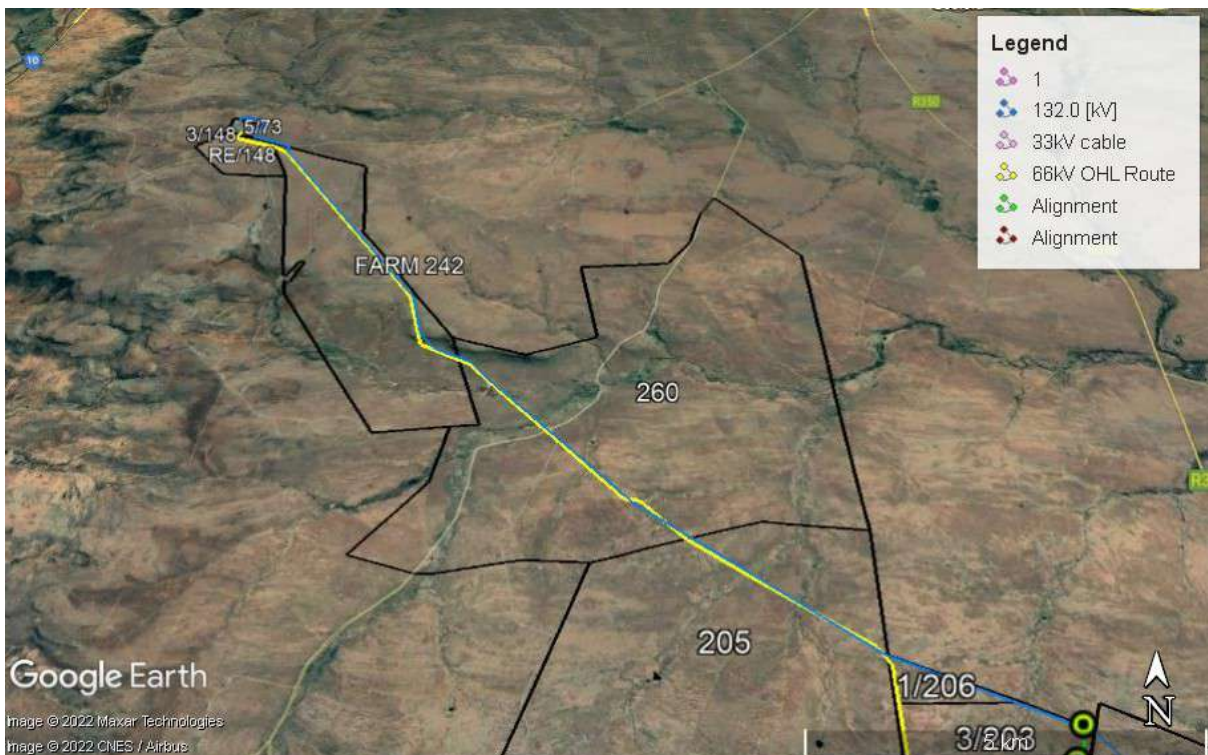
Figure 3: Google Earth map to show the northern part of the 132 kV OHL route for the WEFs - blue line. Yellow line is the existing powerline
