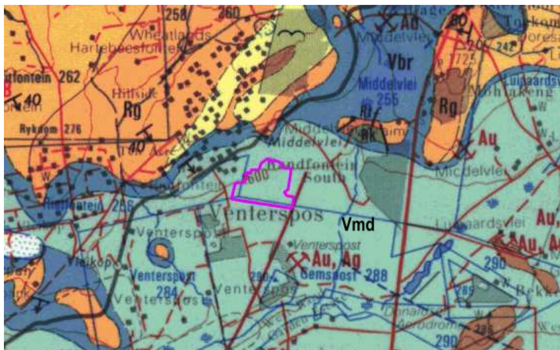
Figure 4: Geological map of the area around the Farm Middelvlei 255 IQ with the project footprint indicated by the lilac outline. Abbreviations of the rock types are explained in Table 2. Map enlarged from the Geological Survey 1: 250 000 map 2626 West Rand.
