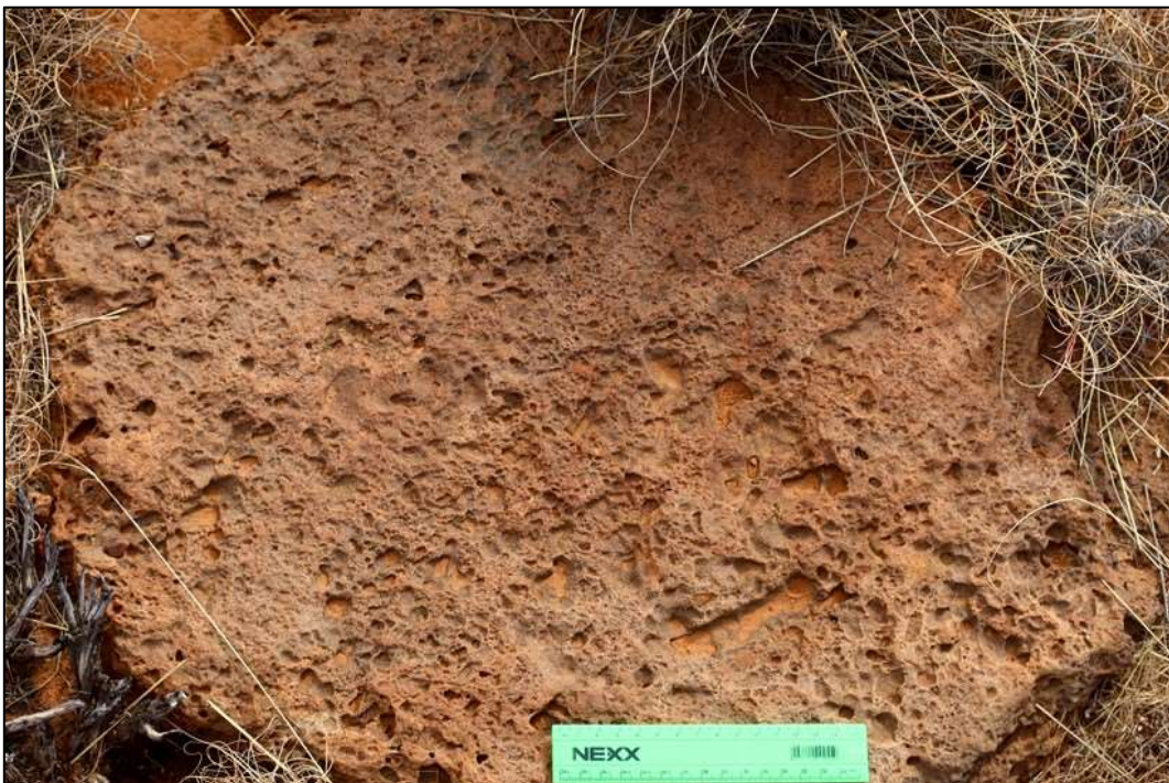
Figure 11: Close-up of channel breccia facies illustrated above showing porous fabric due to dissolution of palaeocalcrete gravel clasts by hot circulating groundwater following dolerite intrusion in the region (Scale = 15 cm). Any reworked fossil bones or teeth originally preserved within the breccias will probably have been dissolved-away at the same time.
