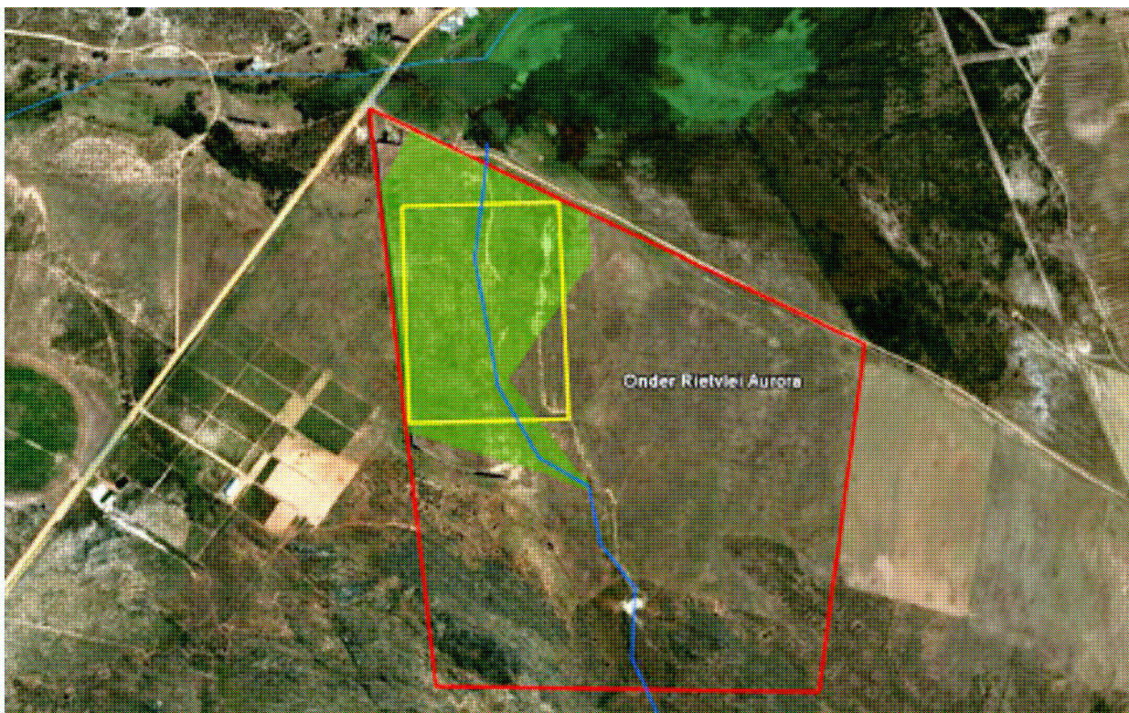
Figure 7: Aerial view of the site with the drainage channel (blue line), proposed layout for the solar panels (yellow rectangle) and estimated area that is seasonally inundated (Belcher 2011: 1)
