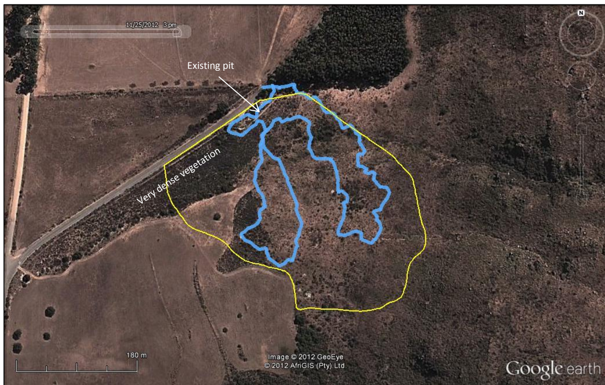
Figure 2: Google earth image showing the polygon of proposed borrow pit 120, the position of the existing borrow pit, the area with very dense vegetation and the author's tracks of the field survey. The tracks of the two assistants which covered other areas were not recorded.
