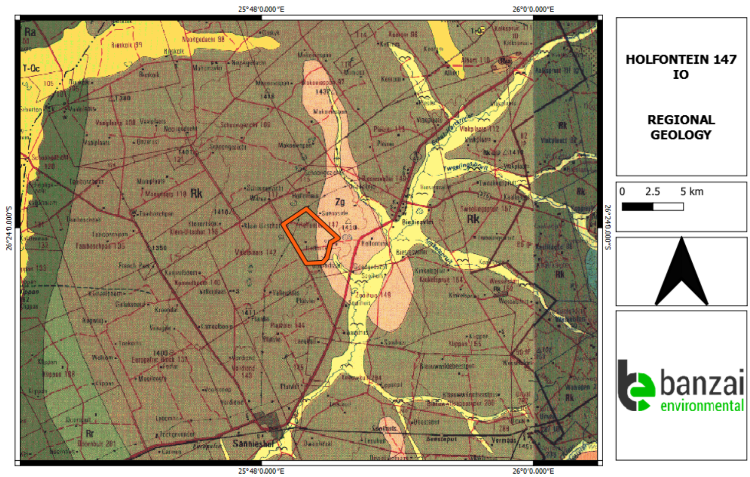
Figure 5: Extract of the 1:250 000 2624 Vryburg Geological map (1992) (Council of Geosciences, Pretoria) indicating the regional geology of the Holfontein drilling site (in orange). The proposed development is underlain by Klipriviersberg Group (Rk) (Ventersdorp Supergroup) and the Kraaipan Group (Zg).
