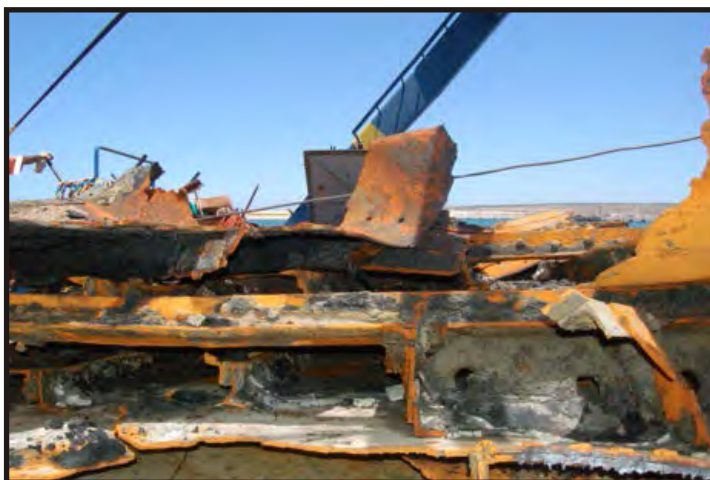
Figure 140 - 141: Seen from the top of the side plating looking down along the frames. The frame and reverse system can be seen. Intercostal plates under certain stringers are also visible. (Photo V. Maitland)
