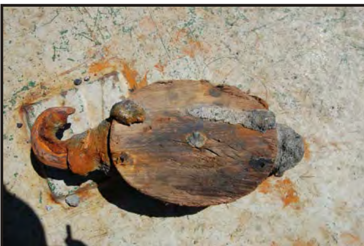
Figure 495: Single, iron strapped block. The hook is shorter and fatter. Unfortunately the conglomerate around the neck of the hook was too thick and I was unable to determine whether the hook could swivel or not. (Photo V. Maitland)
