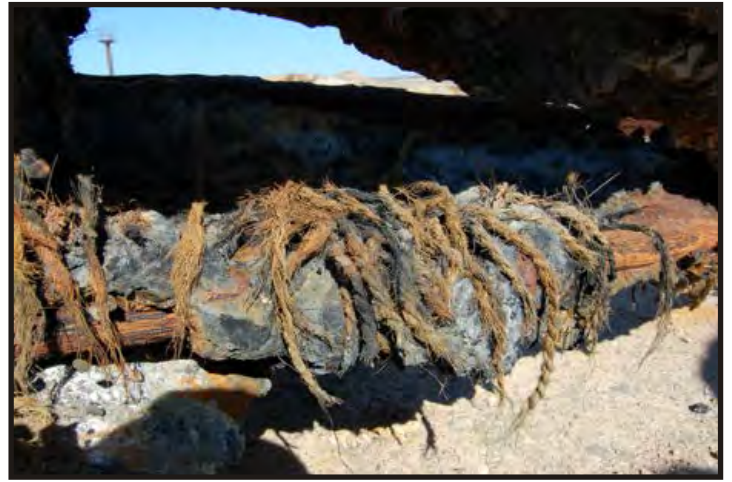
Figure 359 - 360: Strands, ropes and cables were wrapped and lashed on various parts of the wreck. I don't know which were pre-wreck and which were used during the 1904 salvage operation. According to Bisset (1958:93), during quiet times onboard the crew blacked down the rigging. This involved rubbing tar into the rope rigging in order to preserve the manilla (Blackburn 1982:39). (Photo: V. Maitland)
