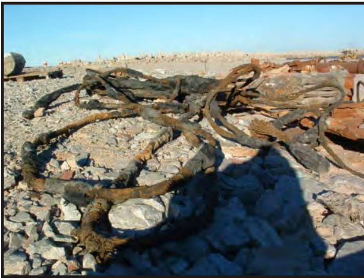
Figure 365: Manilla covered wire rope. (Photo V. Maitland)
