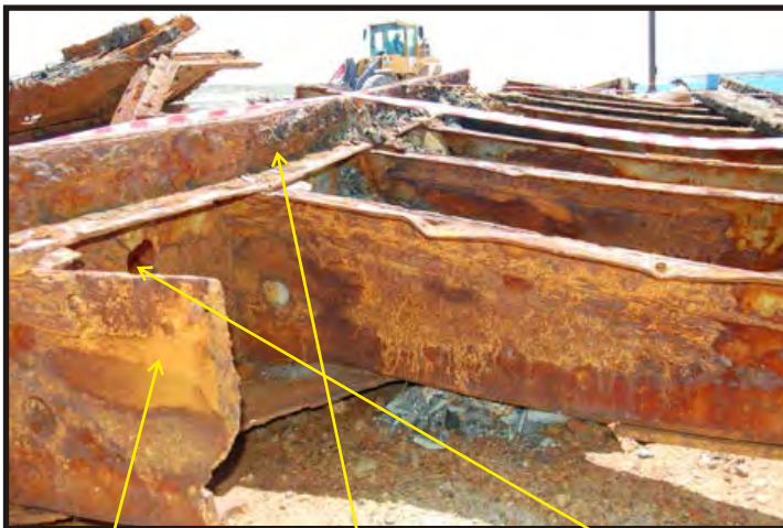
Frames Side Keelson Intercostal Plates
