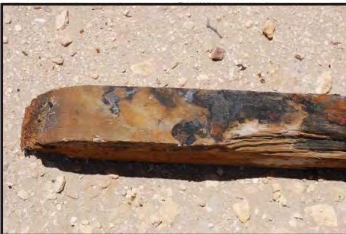
Figure 174: Intercostal block, shaped to fit between the frames. (Photo V. Maitland)
