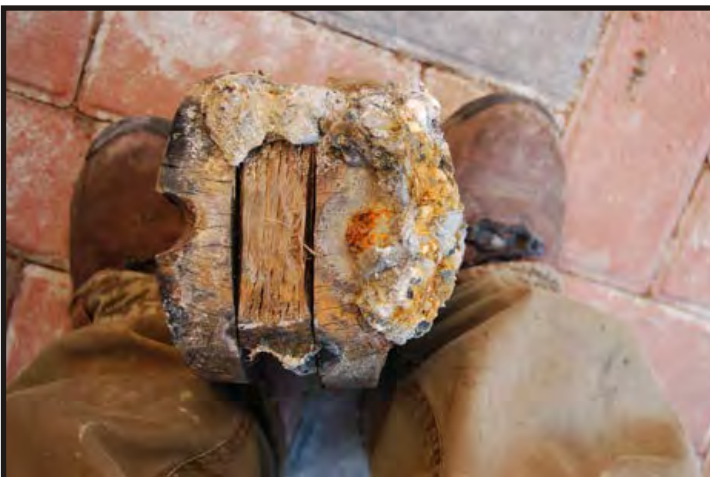
Figure 501: Top view of the scores in the block shell. (Photo V. Maitland)
