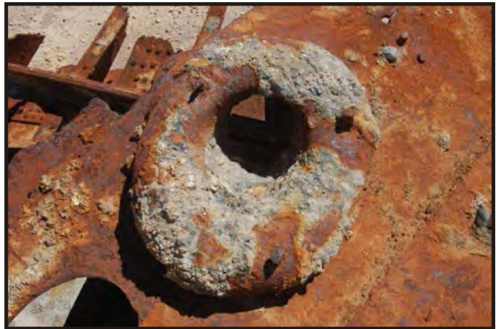
Figure 190: Top view of lower end of hawsepipe as it passed through side plating. There are four rivets attaching it to the plate. (Photo V. Maitland)
