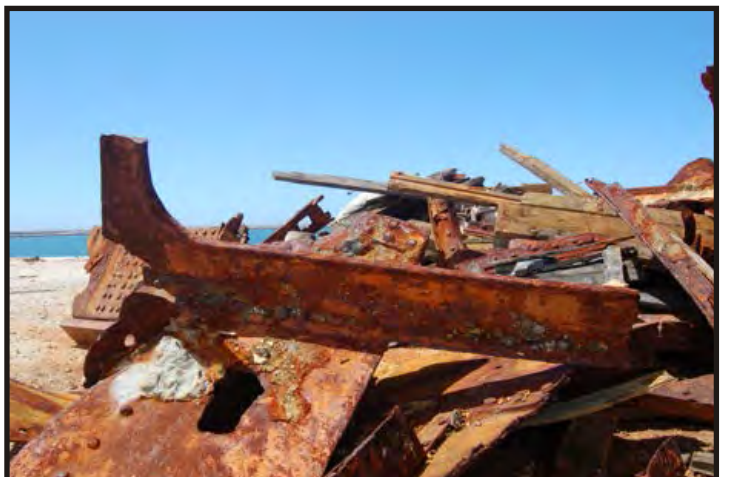
Figure 146: Beam knee, a turned knee with a bulb. (Photo V. Maitland)
