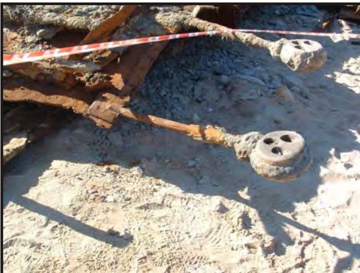
Figure 237: Close-up of the dead-eye attached to the chain plate. (Photo V. Maitland)
