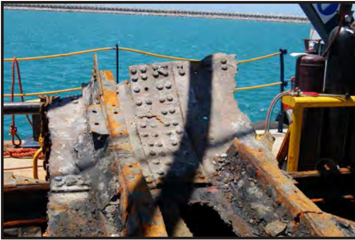
Figure 122: Four rows of chain riveting on a keel butt strap. (Photo V. Maitland)
