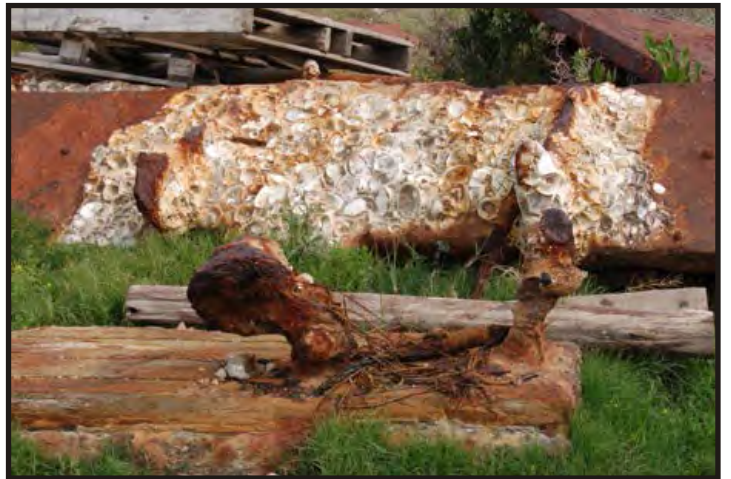
Figures 41 - 42: Corrosion has damaged the head beam further. As it is a fairly substantial piece of iron, human factors have fortunately affected it little. (Photos V. Maitland)
