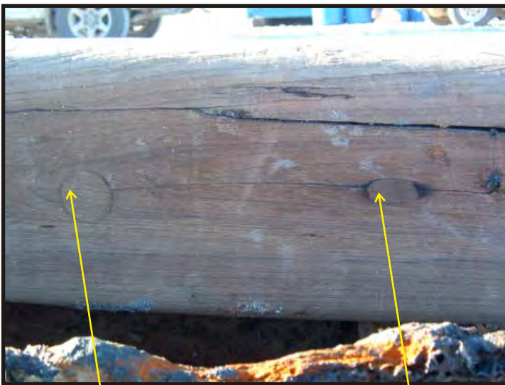
Figure 224: Top of gunwale and dowel covering the bolt, which attaches the gunwale to the supporting angle of the bulwark. Where knots occurred, they were removed and plugged. (Photo V. Maitland)
