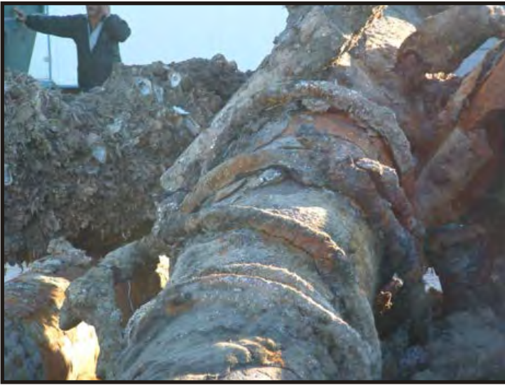
Figure 475: Close-up of cable wrapped around the lower mizzen mast. (Photo V. Maitland)
