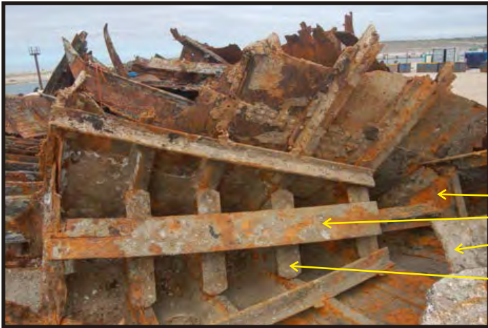
Figure 243: Fore-peak, the narrow part of the vessel's hold close to the bow and under the lowest deck; often only accessible from the general store room (Ward 1891:5). According the Lloyds' Survey of 1881, the County of Pembroke had six breast hooks and five crutches. (Photo V. Maitland)
