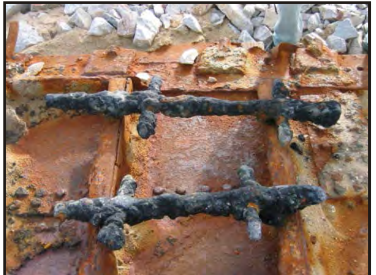
Figure 393 - 394: Railings. The railings around the bow of the barque were known as the pulpit rail. Those in the stern were known as the pushpit or monkey rail. (Photos V. Maitland)
