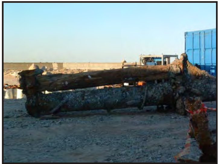
Figure 450: Doubling of the lower iron mast and the wood top mast. The iron trestle trees are still there, but the top is missing. (Photo V. Maitland)
