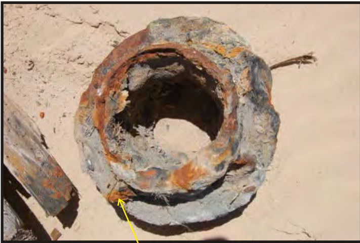
Figure 195: bottom of the upper hawsepipe. A section of the deck planking is visible. (Photo V. Maitland)
