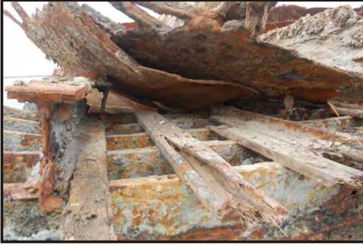
Figure 152: Most vessels have permanent dunnage or a ceiling covering the open floor, it creates space to dry up Maitland) moisture. (Brown 1931:391; Photo V. Maitland)
