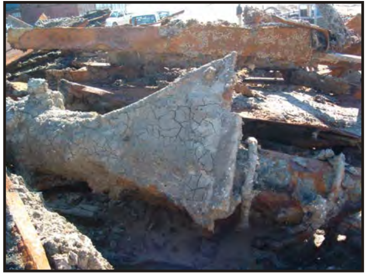
Figure 476: Close-up of cheeks under the top of the lower mizzen mast. (Photo V. Maitland)
