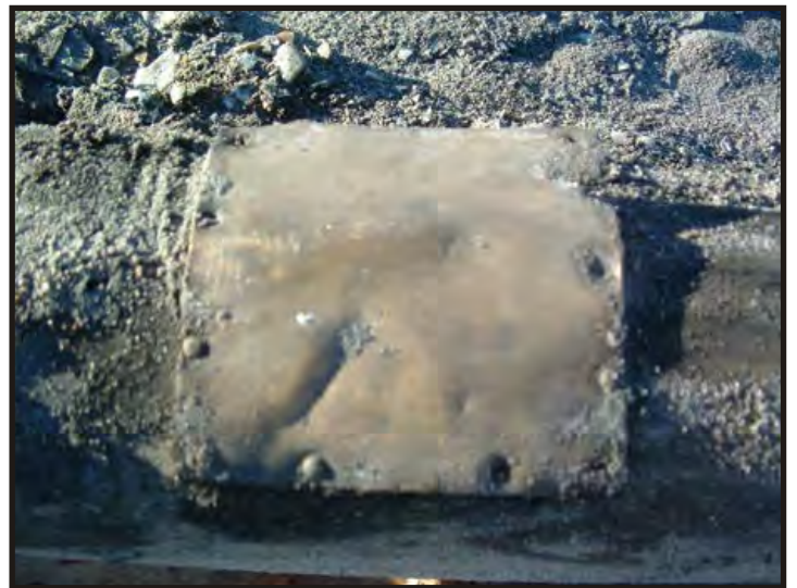
Figure 227: Top of gunwale. Repairs were made to the wood and covered with a copper sheet. (Photo V. Maitland)
