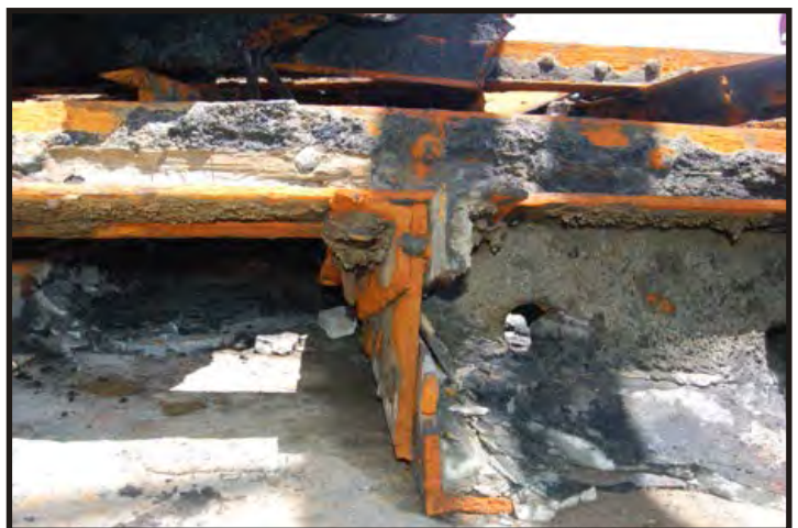
Figure 140 - 141: Seen from the top of the side plating looking down along the frames. The frame and reverse system can be seen. Intercostal plates under certain stringers are also visible. (Photo V. Maitland)
