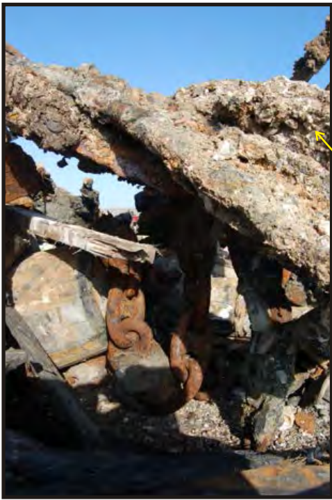
Figure 349 - 350: Bower cable. According to the Lloyds' Survey of 1881, the County of Pembroke had 270 fathoms of 1¾" chain. The Eastern Province Herald (27-11-1903), states the County of Pembroke had two chains of 135 fathoms each and 1¾ inches in thickness, this tallies with the Lloyds' Survey. In Figure 349, it appears that there is a hawse pipe or a spurling pipe above where the chain is attached to the beam. Figure 350 is a close-up of the beam attachment. (Photos V. Maitland)
