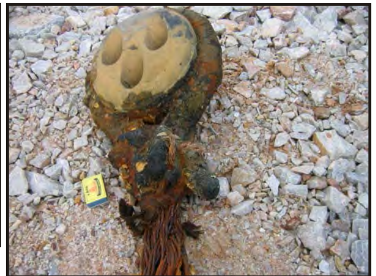
Figure 490: Close-up of dead-eye. Iron wire cable is in the groove. (Photo V. Maitland)
