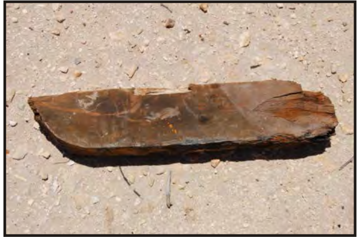
Figure 173: Intercostal block, shaped to fit between the frames. (Photo V. Maitland)
