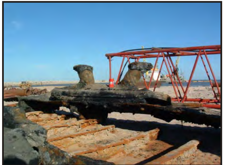
Figure 312 - 313: Bollards are stout vertical posts used for securing the lines when a ship is moored. They usually appear in pairs sharing the same base, which is fixed to the vessel rather than being an integral part of the vessel as are the bitts, which are often used for the same purpose (Blackburn 1981:44). These bollards were made of cast iron and they attached to a shaped wooden piece; this in turn was attached to the deck planking, which was attached to the rider plate. (Photos . V. Maitland)
