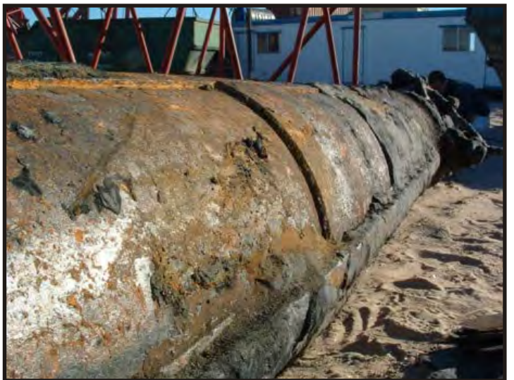
Figure 458: Different view of the lower main mast and clasp hoops. (Photo V. Maitland)
