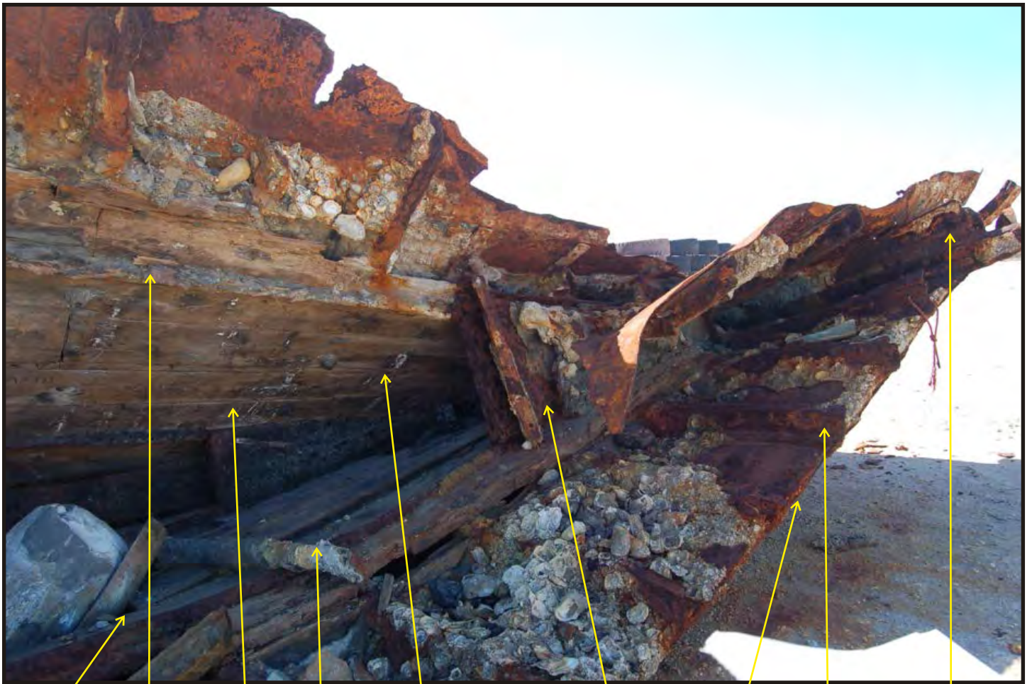
Port Side Stringer Ceiling Pillar Starboard Rider Plate Side Plating Frame Stern-post
