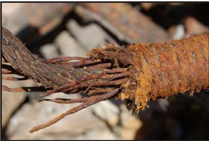
Figure 361 - 362: Wire rope. According to the Manual of Seamanship (1951:89), wire rope consists of many small wires extending continuously throughout its length, these are twisted into strands; the strands are twisted around a jute or hemp heart. The wire ropes from the County of Pembroke were wrapped with manilla, hemp or jute. The heart acts as a cushion into which the strands bed, giving the rope more flexibility. The heart and covering absorbs the oils with which the ropes are treated. As the ropes are stretched or flexed, the oils are squeezed between the wires lubricating them and reducing friction. According to Bisset (1956: 214) slush was mixed with Stockholm tar for greasing down the rigging, masts and for splicing ropes. (Photos V. Maitland)
