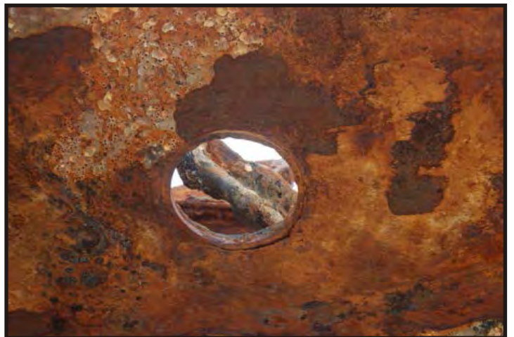
Figure 198: Close-up of inner side of the porthole. The correct terms for a porthole are deadlight or scuttle. (Blackburn 1981:243; Photo V. Maitland)
