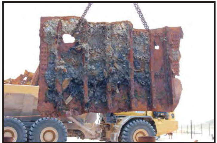
Figure 108: Side plating showing the frames and two butt straps. (Photo V. Maitland)
