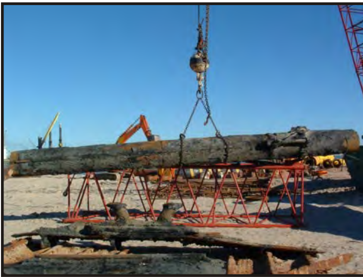
Figure 455: Lower main mast. The bottom of the mast, just above the partners, is ringed with cleats. (Photo V. Maitland)
