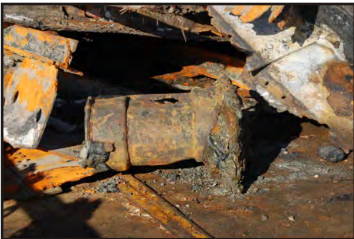
Figure 373: Pump. Two of these were found. This is the discharge end of the pump. According to the Lloyds' Survey of 1881, the County of Pembroke had two metal chambered pumps aboard. Bisset (1958:52,201) states that the fresh water was stored in two iron tanks set amidships in the hold. Water was drawn with a hand pump on deck into buckets. The ration per man per day was three quarts. The other pump may have been a bilge pump. (Photo V. Maitland)
