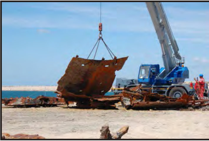
Figure 106: Section of side plating. At the upper edge of the plating, note the in-and-out system. (Photo: V. Maitland)
