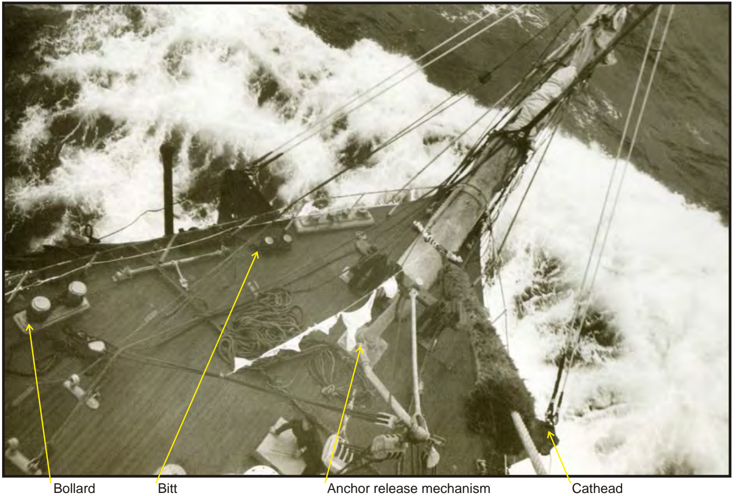
Figure 311: View from the foremast looking down to the foredeck and bowsprit of the Lawhill . The anchor release mechanism is between the bitts and bollards on each side. Catheads can be seen on either side. (Spencer 1997:21; Photo G. Belton)
