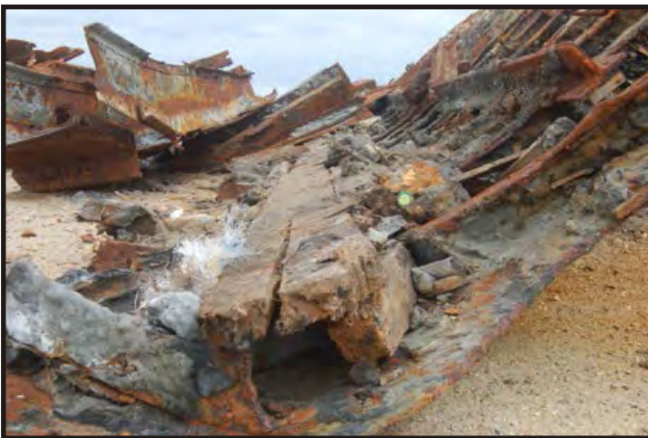
Figure 168: Turn of the bilge, showing the ceiling. (Photo V. Maitland)
