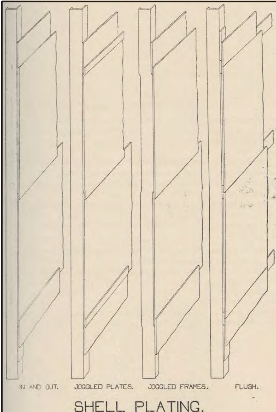
Figure 105: Diagram of shell plating. In-and-out plating gradually gave way to joggled plating. In-and-out plating requires liners to be fitted between the out-strakes and the frames to give a proper connection. (Pursey 1942:82; Drawing H.J. Pursey)
