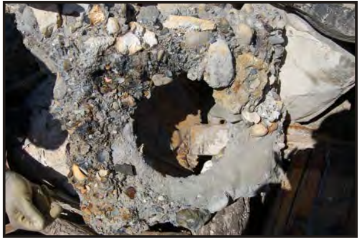
Figure 194: Top view of upper end of hawsepipe, this was riveted to the deck. (Photo V. Maitland)
