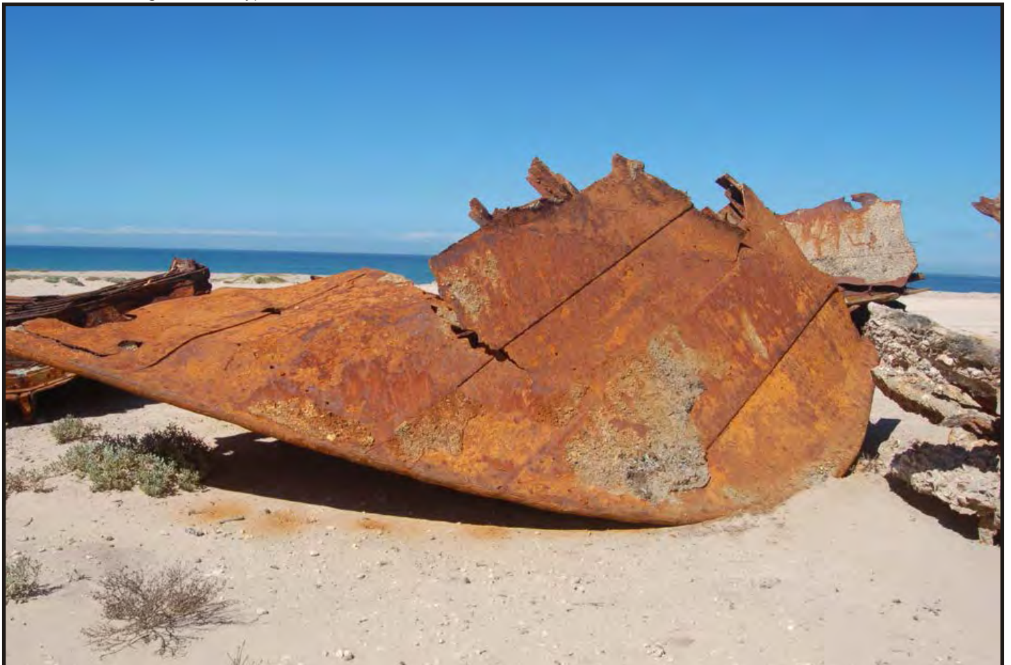
Figure 240: Bottom of the bow of the County of Pembroke . (Photo V. Maitland)
