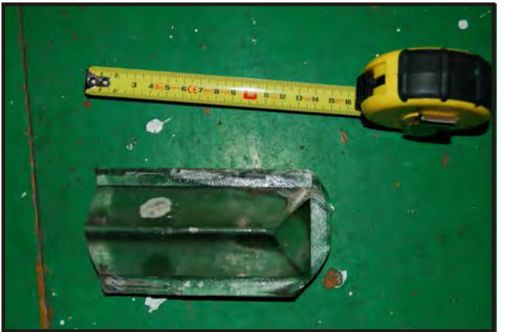
Figure 397 - 398: Figure 397, deck side of a piece of skylight. Figure 398 is the underside. (Photos V. Maitland) On the voyage to Australia in November 1898, 300 miles to the south of the Cape of Good Hope, the County of Pembroke was running before a gale and had heaved to in order to wait for the wind to drop a little. A gigantic wave crashed from astern onto the poop and the wave stoved in and carried away the teakwood, glass cabin skylight, companionway and binnacle. Water flooded the compartments and alleyways under the poop. The ship came very close to being sunk and all hands set to repair the damages, batten down the holes and save whatever stores they could. The flooded areas were bailed out with buckets hauled up on lines (Bisset 1958:84-87).
