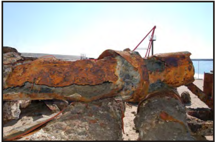
Figure 448: Section of mast with the wedge strap, this was a doubling of the mast where it went through the deck. (Photo V. Maitland)
