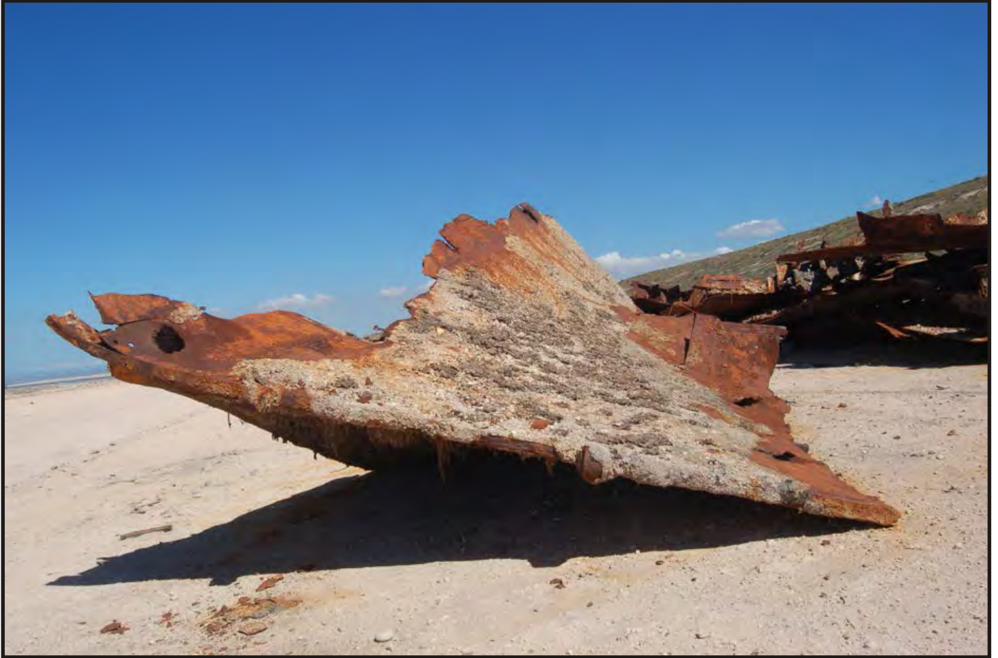
Figure 260: Stern. Gudgeons are on the rudder post and pintles fitted into the gudgeons. According to the Lloyds' Survey of 1881, the stern post is the same dimensions as the keel and stem. Unfortunately the keel was not attached to the stern.
