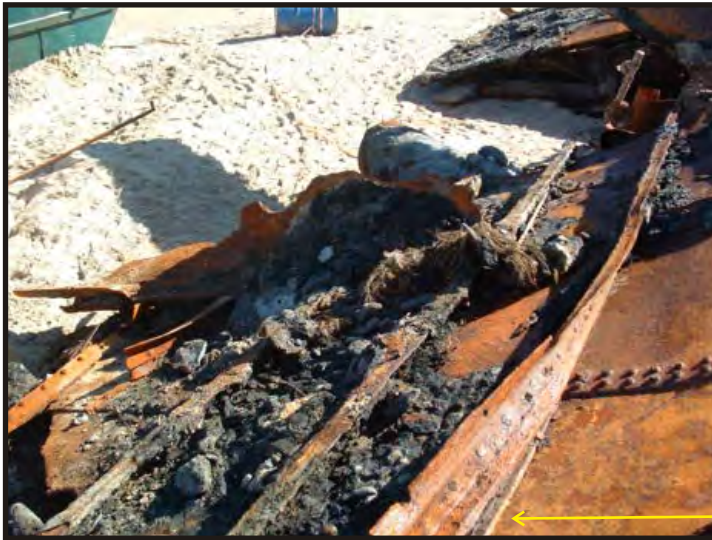
Figure 113 - 114: Frames on the side plating. A liner had to be fitted under the frames to ensure a proper connection between the out stakes and frames. (Photo V. Maitland)
