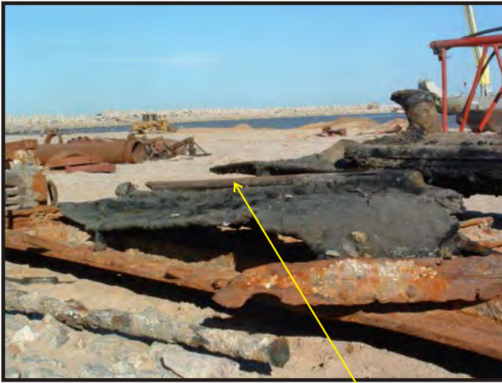
Figure 222: Bulwark, seen from bottom. Note gunwale at the back. (Photo V. Maitland)
