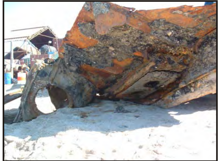
Figure 196: Bottom of starboard bow hawsepipes. Most vessels had three hawsepipes on the bow, one on the port and two on the starboard side. One on each side is for the bower anchors, the second one on the starboard side is for the sheet anchor (Blackburn 1981:157; Photo V. Maitland)
