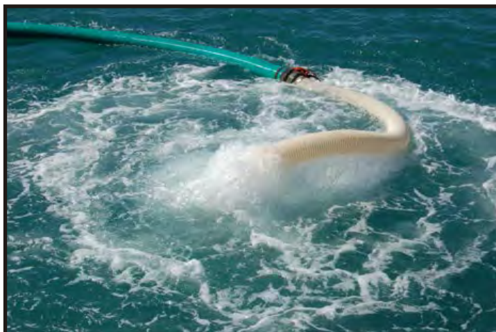
Figures 51 - 52: The dredge hose is used to remove silt overburden from the wreck. The grid on the front prevents large objects from being sucked up. (Photos V. Maitland)
