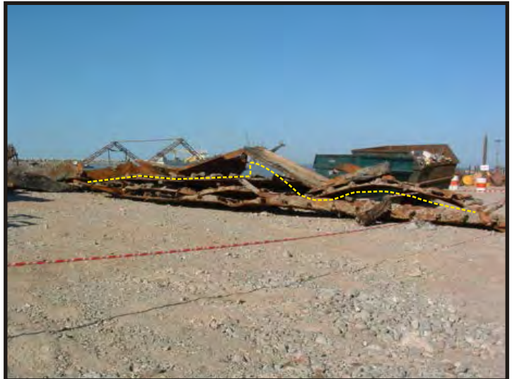
Figure 219: Long section of the bulwark removed in 2004. The supporting angle of the gunwale is towards us. (Photo V. Maitland)
