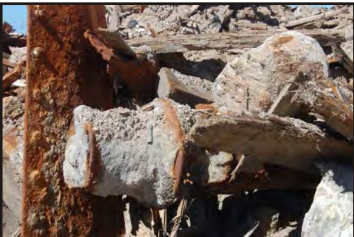
Figure 326: Drum end of windlass. Directly to the right of the drum is a gypsy. (Photo V. Maitland)
