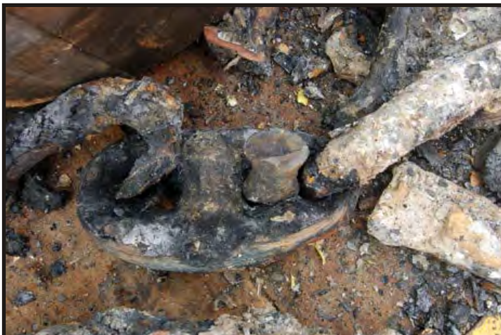
Figure 353: Chain links with a stud in the links. (Photo V. Maitland)
