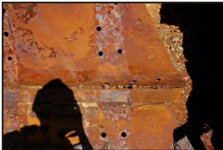
Figure 102: Keel from above, showing where the frames were riveted to the garboard strake. (Photo V. Maitland)
