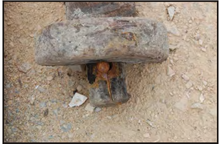
Figure 426: Close-up of wooden axle and wheel showing the pin holding the wheel on. (Photo V. Maitland)
