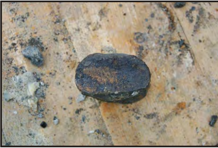
Figure 355: Close-up of the top of the chain stud. Studs were fitted in the links to keep the chain from kinking and added strength to the chain. (Brown 1931:119; Photo V. Maitland)
