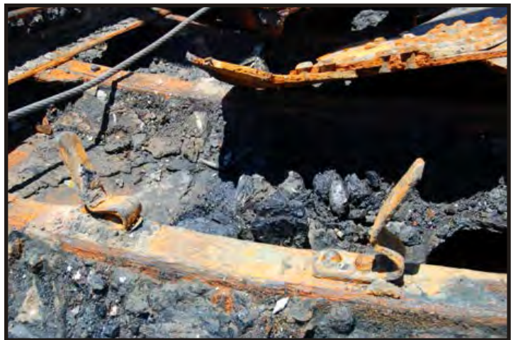
Figure 169: Cleats on side frames. These hold the side battens, which are part of the hold ceiling. This permanent dunnage is sufficient for rough cargoes and other goods not liable to absorb moisture. (Brown 1931:391; Photo V. Maitland)
