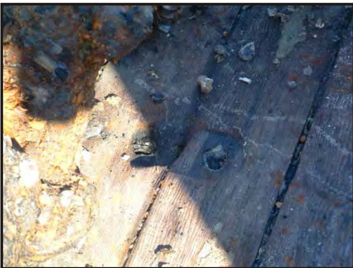
Figure 387: Imprint and bolts of deck rigging or equipment. (Photo V. Maitland)
