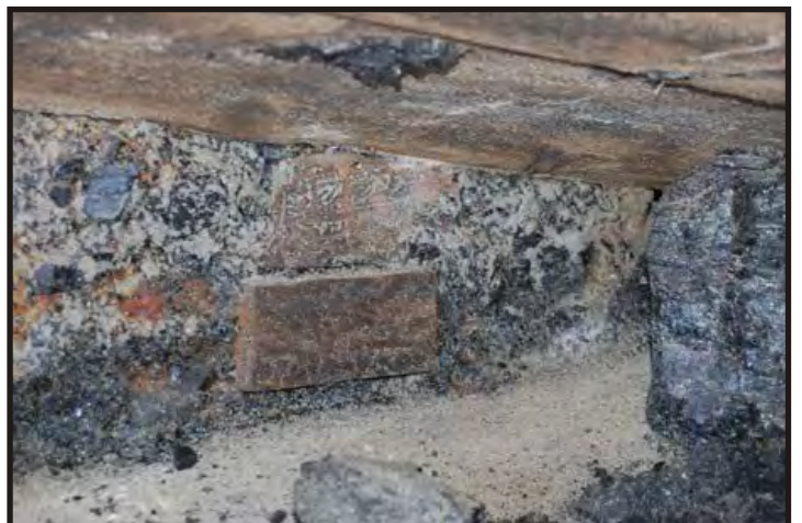
Figure 269: Close-up of rudder-post area and top of the lower rider plate. The coal was part of the cargo. The wood may have been temporary dunnage. (Photo V. Maitland)
