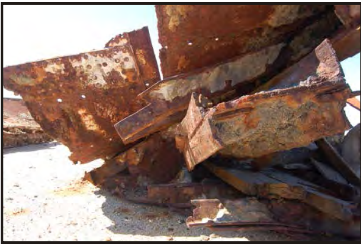
Figure 264: Close-up of the keel section of the stern. The keel is gone, the keelson is still visible. (Photo V. Maitland)
