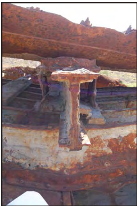
Figure 443: Centre keelson and mast step. The downward thrust that a mast exerts at its heel means the mast must be strongly supported and stepped (Pursey 1942:144). By putting the mast through the decks, it added support to the mast. In the County of Pembroke the mast was stepped on the centre keelson; it had a reinforcing bracket where it's wider than the keelson. (Photo V. Maitland)
