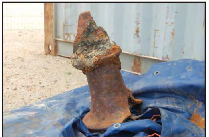
Figure 333: This may either be a drum end of a windlass or a winch, which is a small vertical drum around which a rope or line is passed in order to make it easier to pull the rope. The principle difference between the two, is a windlass is horizontally mounted on the deck while a winch is vertically mounted and is an integral part of the deck. (Blackburn 1981:341; Photo V. Maitland)
