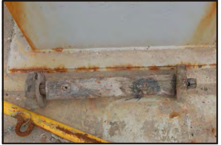
Figure 424: Wooden axle and wheels, probably from a deck trolley. The remains of iron bolts on the axle are visible. (Photo V. Maitland)
