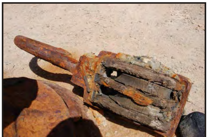
Figure 496: Double, iron strapped block. The large hook appears to hinge onto the iron strap and was probably able to pivot. The iron strap is still in place. (Photo V. Maitland)
