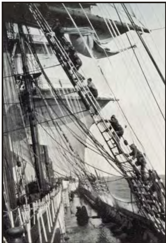
Figure 437: Scrambling up the shrouds to work on the masts, yards or sails (Villiers 1933:32). Aboard the County of Pembroke most of the lines for handling sail were belayed along the rail, amidships (Bisset 1958:82).
