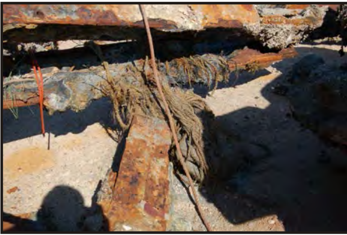
Figure 359 - 360: Strands, ropes and cables were wrapped and lashed on various parts of the wreck. I don't know which were pre-wreck and which were used during the 1904 salvage operation. According to Bisset (1958:93), during quiet times onboard the crew blacked down the rigging. This involved rubbing tar into the rope rigging in order to preserve the manilla (Blackburn 1982:39). (Photo: V. Maitland)
