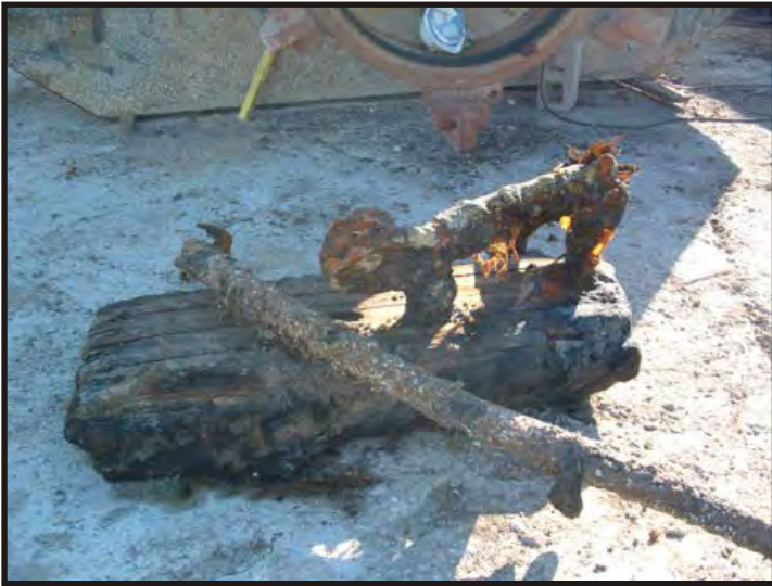
Figures 43 - 44: This rigging gear has become severely damaged in the last three years. It collapsed in places as the rust ate into the core metal. (Photos V. Maitland)
