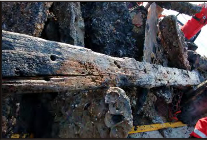
Figure 217: Deck plank. This is different from the other planks, it has several rows of three holes each for fasteners; it could be from a different part of the barque or from another wreck. It is possible that when the wreck was removed from North End Beach, the salvors loaded parts of other wrecks onto the County of Pembroke to clean up the problems that wrecks were causing. (Photo V. Maitland)
