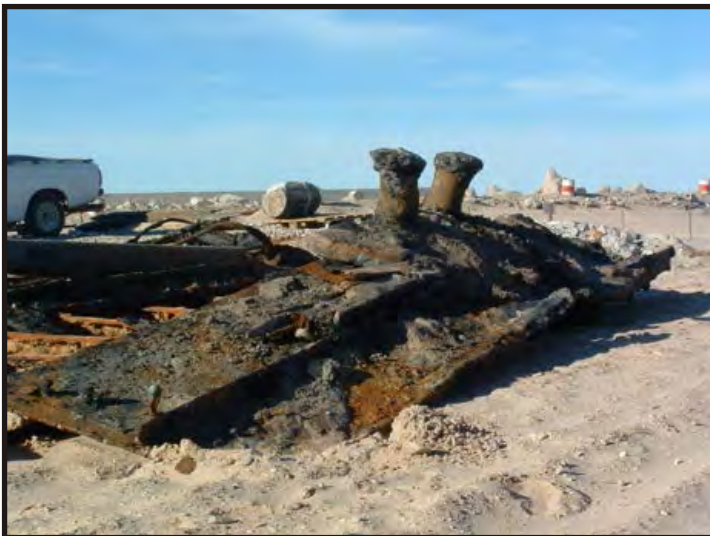
Figure 312 - 313: Bollards are stout vertical posts used for securing the lines when a ship is moored. They usually appear in pairs sharing the same base, which is fixed to the vessel rather than being an integral part of the vessel as are the bitts, which are often used for the same purpose (Blackburn 1981:44). These bollards were made of cast iron and they attached to a shaped wooden piece; this in turn was attached to the deck planking, which was attached to the rider plate. (Photos . V. Maitland)
