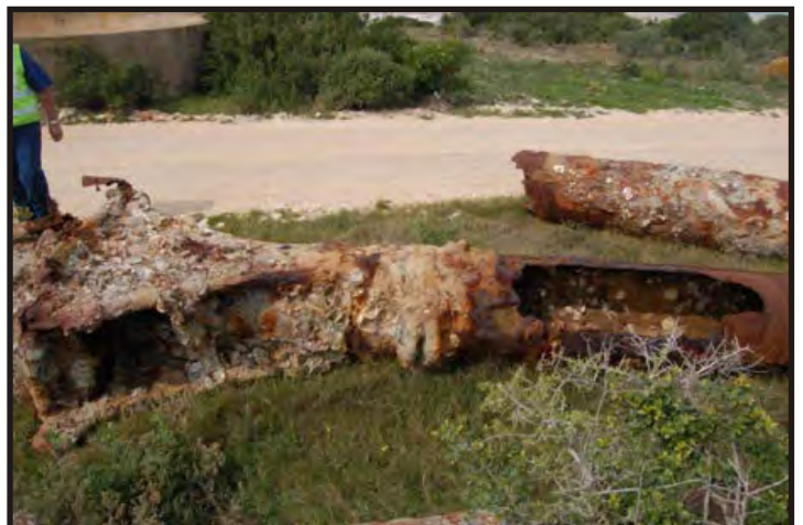
Figures 453 - 454: Two different views of the trestle trees and doubling of the mast. (Photo V. Maitland)
