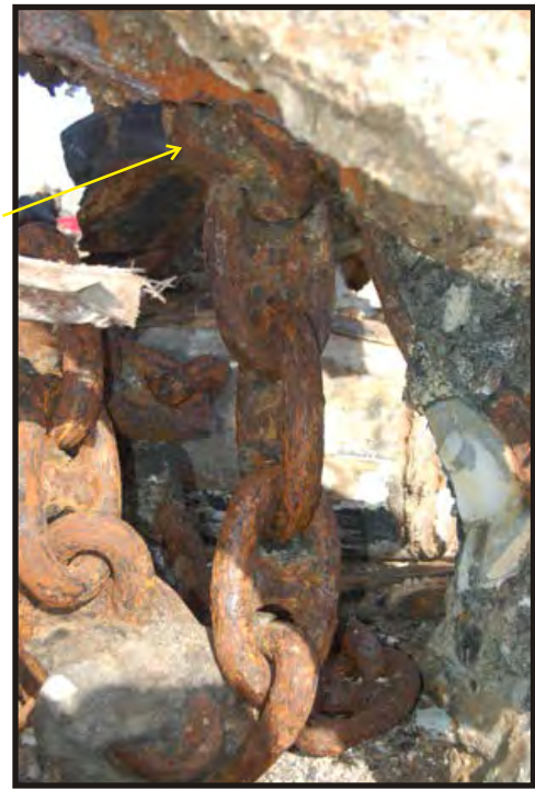
Figure 349 - 350: Bower cable. According to the Lloyds' Survey of 1881, the County of Pembroke had 270 fathoms of 1¾" chain. The Eastern Province Herald (27-11-1903), states the County of Pembroke had two chains of 135 fathoms each and 1¾ inches in thickness, this tallies with the Lloyds' Survey. In Figure 349, it appears that there is a hawse pipe or a spurling pipe above where the chain is attached to the beam. Figure 350 is a close-up of the beam attachment. (Photos V. Maitland)
