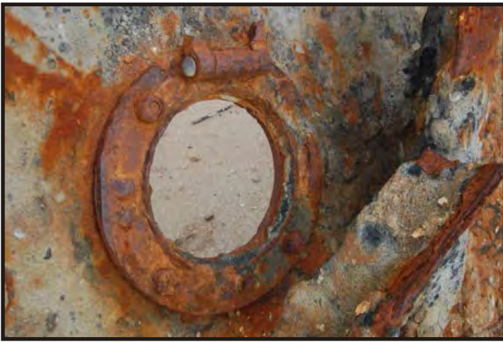
Figure 199: Close-up of a stern porthole. It still has the frame riveted to the plating. (Photo V. Maitland)
