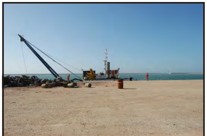
Figure 83: When the deck of the barge is full and all the bins have been lifted off the wreck, the barge is brought alongside and the artefacts hoisted onto the quay. (Photo V. Maitland)
