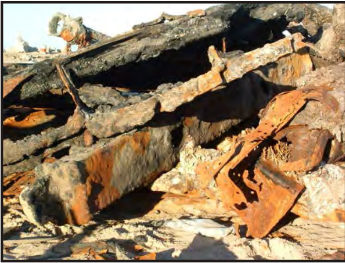
Figures 41 - 42: Corrosion has damaged the head beam further. As it is a fairly substantial piece of iron, human factors have fortunately affected it little. (Photos V. Maitland)
