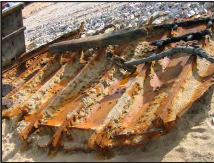
Figures 37 - 38: While the materials appear to be as coated with rust in 2004 as they are in 2007, in 2004 it was a light layer over an unaffected core. After three years the rust had eaten into the iron and is corroded the core. The onion-peel look bears this out. In addition, all the dead-eyes have been removed by persons unknown. (Photos V. Maitland)
