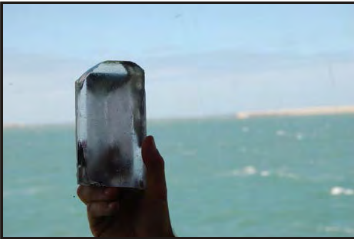
Figure 397 - 398: Figure 397, deck side of a piece of skylight. Figure 398 is the underside. (Photos V. Maitland) On the voyage to Australia in November 1898, 300 miles to the south of the Cape of Good Hope, the County of Pembroke was running before a gale and had heaved to in order to wait for the wind to drop a little. A gigantic wave crashed from astern onto the poop and the wave stoved in and carried away the teakwood, glass cabin skylight, companionway and binnacle. Water flooded the compartments and alleyways under the poop. The ship came very close to being sunk and all hands set to repair the damages, batten down the holes and save whatever stores they could. The flooded areas were bailed out with buckets hauled up on lines (Bisset 1958:84-87).
