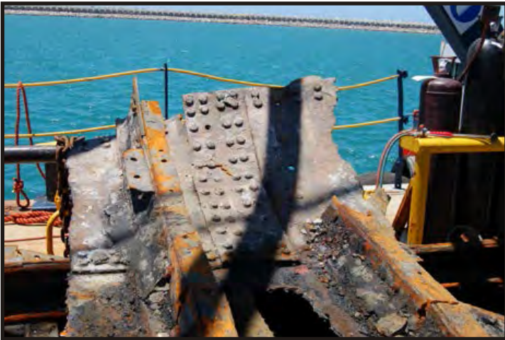
Figure 133: Turn of the bilge and floor head. (Photo V. Maitland)
