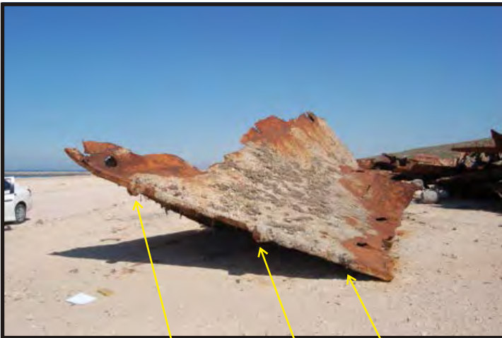
Figure 307: Rudder post with three gudgeons. These are eyes into which the rudder pintles fit. (Blackburn 1981:148; Photo V. Maitland)
