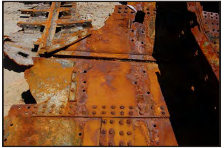
Figure 112: Section of the keel, garboard strake and keel strake with a butt strap. The joints are staggered to strengthen the hull. (Photo V. Maitland)
