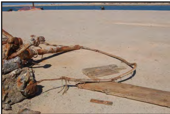
Figure 487: Dead-eyes in the channel on the bulwarks. (Photo V. Maitland)
