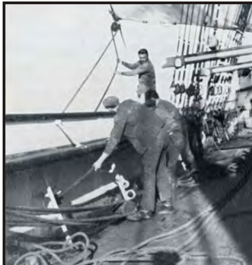
Figure 219: Long section of the bulwark removed in 2004. The supporting angle of the gunwale is towards us. (Photo V. Maitland)
