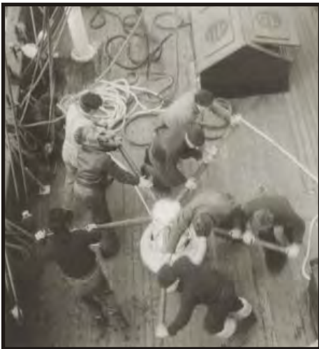
Figure 337 : Men trudging around the capstan aboard the Lawhill . (Spencer 1997:20; Photo G. Belton)
