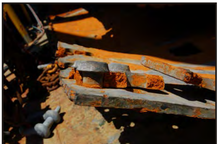
Figure 119: Side view of pan head rivets; the taper of the rivet can be seen. (Photo V. Maitland)
