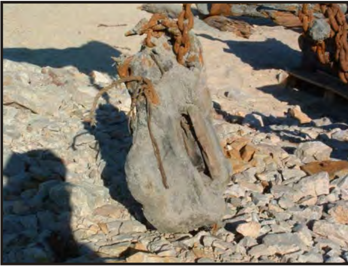
Figure 472: Close-up of the double block attached to the trunnion hoop of the lower main mast. (Photo V. Maitland)
