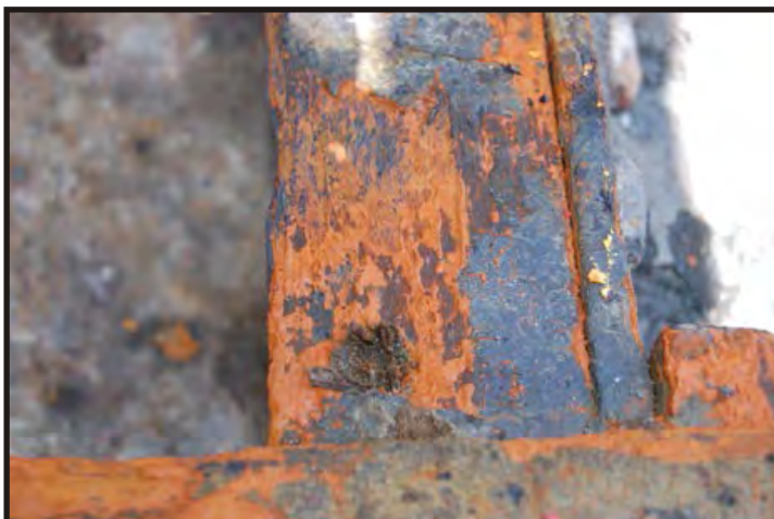
Figure 156: Top view of wooden dowel. The ceiling on the keel floor was attached with wooden dowels. (Photo V. Maitland)
