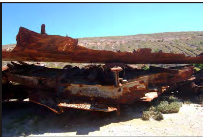
Figure 135: The County of Pembroke had a bar keel. The keelson is a built H-beam, running fore and aft, it has a rider plate above it. There are four side keelsons, two per side. There are two bilge keelsons, these are the precursors to brackets and add strength. (Photo V. Maitland)
