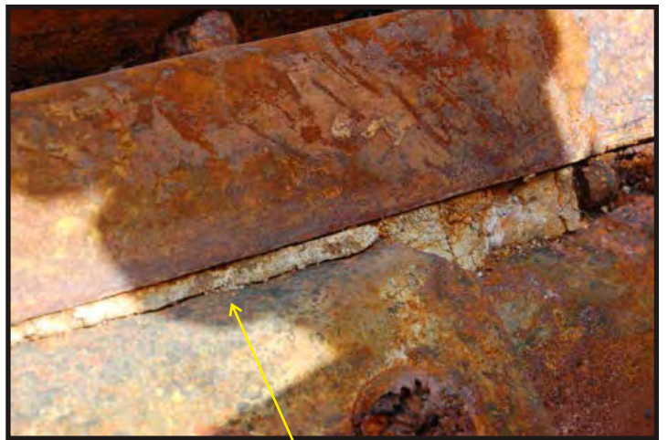
Figure 124 - 125: The Lloyds' Survey of 1881 states that the inside surfaces of the barque were protected from oxidation by cement and paint. Joints in the keel were usually caulked, this operation had to be carefully done. If the caulking was pushed too far into the joint it could cause it to separate, and if not pushed in enough, would not provide a watertight seal. (Pursey 1942:16) The cement caulking can be seen covering the web frame in Figure 124 and in the join of the bar keel to the garboard strake in Figure 125. (Photos V. Maitland)
