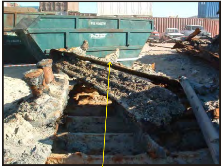
Figure 234: Bulwark. Where there are no channels the stanchion is different, it's a solid bracket. (Photo V. Maitland)
