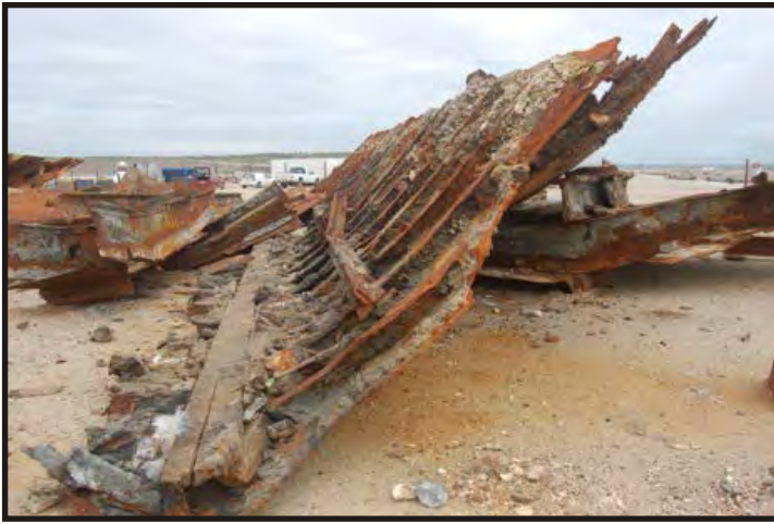
Figure 142: Side stringers add longitudinal strength to the hull. (Photo V. Maitland)
