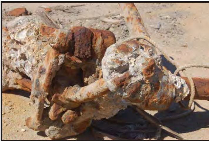
Figure 379: Close-up of cog on the possible anchor release mechanism. (Photo V. Maitland)
