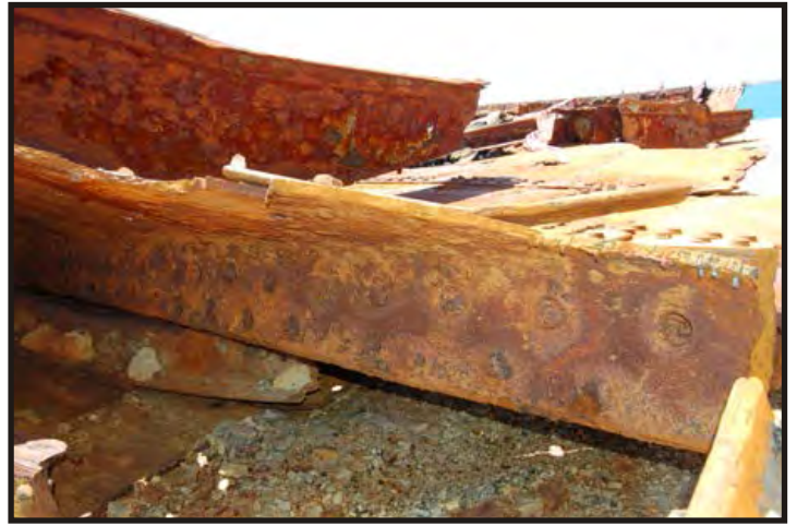
Figure 104: Zig-zag riveting of the garboard strake to the bar keel. (Photo V. Maitland)
