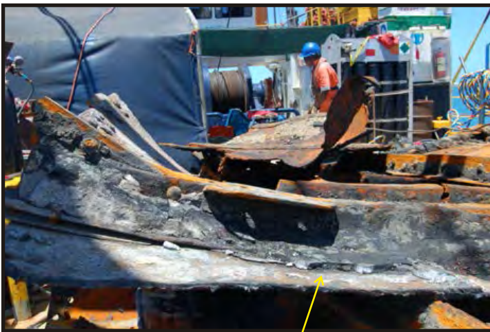
Figure 124 - 125: The Lloyds' Survey of 1881 states that the inside surfaces of the barque were protected from oxidation by cement and paint. Joints in the keel were usually caulked, this operation had to be carefully done. If the caulking was pushed too far into the joint it could cause it to separate, and if not pushed in enough, would not provide a watertight seal. (Pursey 1942:16) The cement caulking can be seen covering the web frame in Figure 124 and in the join of the bar keel to the garboard strake in Figure 125. (Photos V. Maitland)
