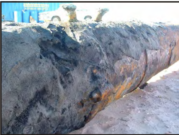
Figure 457: Lower main mast showing the clasp hoops, these are strong circles of iron driven onto masts with a hinge in the middle fastened together with forelocks through mortises (Steel 1794:6). (Photo V. Maitland)
