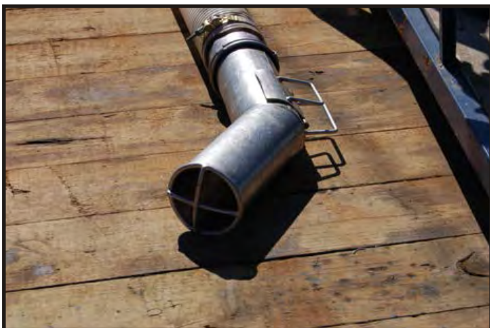
Figures 51 - 52: The dredge hose is used to remove silt overburden from the wreck. The grid on the front prevents large objects from being sucked up. (Photos V. Maitland)
