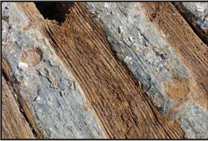
Figure 211: Close-up of the deck. The wooden dowels are visible. According to Bisset (1958:67) when the ship was stuck in the doldrums, the pitch in the deck seams softened and the crew had to haul up buckets of sea water to douse the decks. (Photo V. Maitland)
