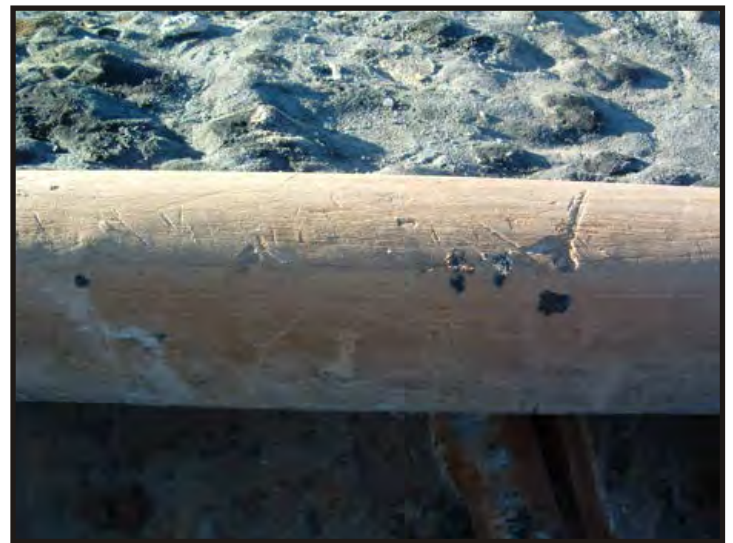
Figure 225: Close-up of the gunwale, nicks and scratches from shipboard work visible. (Photo V. Maitland)
