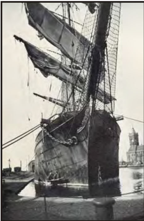
Figure 341: Bows of the iron sailing vessel, Wanderer . The cathead holding the anchor at the bulwark can be seen with the anchor cable in the hawsepipe. (Villiers 1933:224)
