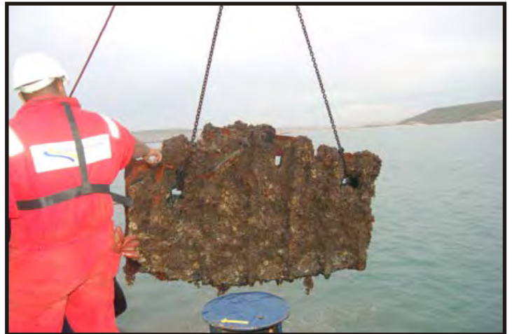
Figure 81: 2 x 3m section of side plating. The hull was cut underwater using broder rods and then lifted onto the deck of the Ubejane . (Photo V. Maitland)
