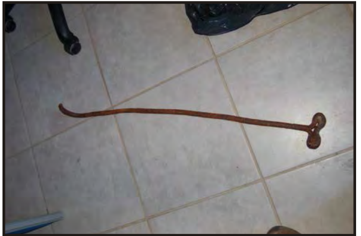
Figure 421: Chain-hook. (Photo V. Maitland) According to Luce (1891:276) hook ropes are single ropes with a hook on one side. These were used in lighting along the chain in conjunction with the above long handled chain-hook.
