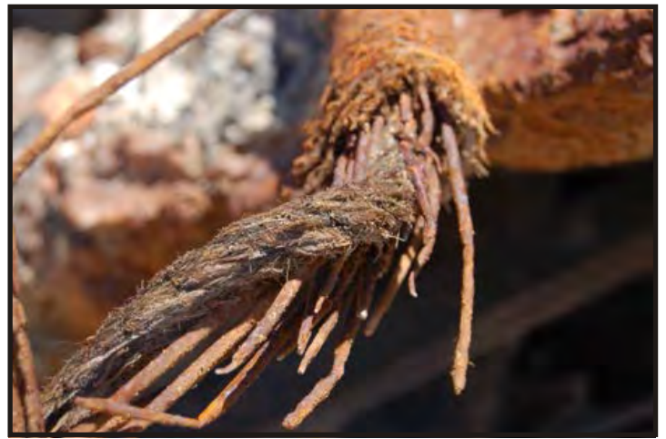
Figure 361 - 362: Wire rope. According to the Manual of Seamanship (1951:89), wire rope consists of many small wires extending continuously throughout its length, these are twisted into strands; the strands are twisted around a jute or hemp heart. The wire ropes from the County of Pembroke were wrapped with manilla, hemp or jute. The heart acts as a cushion into which the strands bed, giving the rope more flexibility. The heart and covering absorbs the oils with which the ropes are treated. As the ropes are stretched or flexed, the oils are squeezed between the wires lubricating them and reducing friction. According to Bisset (1956: 214) slush was mixed with Stockholm tar for greasing down the rigging, masts and for splicing ropes. (Photos V. Maitland)
