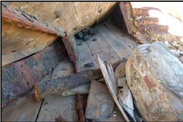
Figure 266: Close-up from the side towards the rudder-post. The keelson can be seen running under the two rider plates. (Photo V. Maitland)
