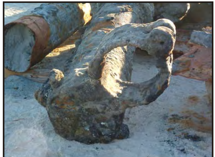
Figure 480: Close-up of lower mizzen mast cap and trunnion hoop. (Photo V. Maitland)
