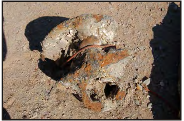
Figure 329: Close-up of gypsy, part of the windlass. (Photo V. Maitland)
