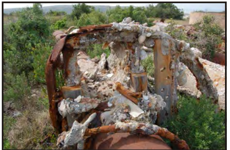
Figures 37 - 38: While the materials appear to be as coated with rust in 2004 as they are in 2007, in 2004 it was a light layer over an unaffected core. After three years the rust had eaten into the iron and is corroded the core. The onion-peel look bears this out. In addition, all the dead-eyes have been removed by persons unknown. (Photos V. Maitland)
