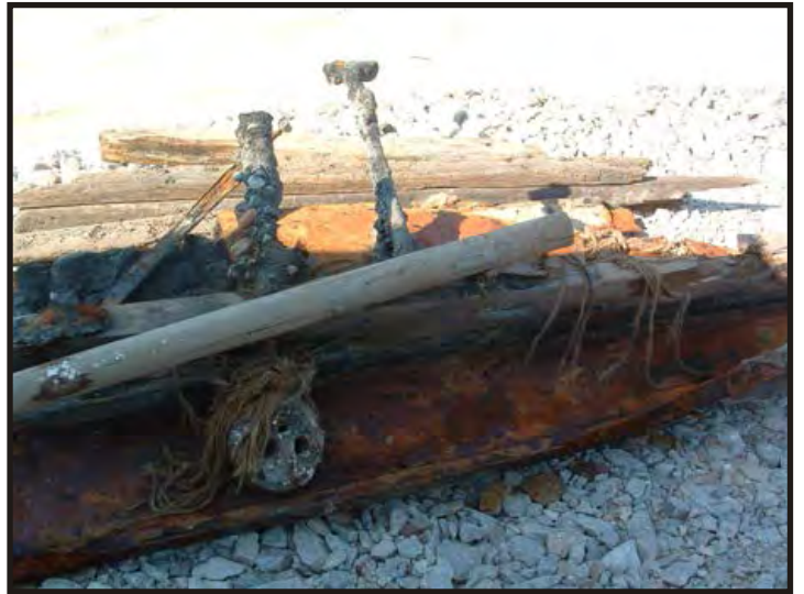
Figure 230: Channel showing a stanchion and dead-eye. Cordage is tangled around the dead-eye. (Photo V. Maitland)
