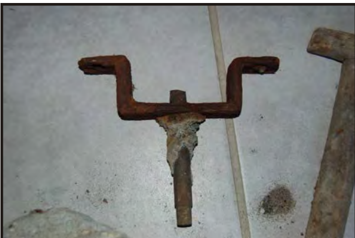
Figure 416: Iron and brass fastener. (Photo V. Maitland)
