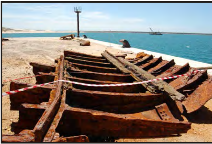
Figure 131: There are no brackets in the bilge in keeping with earlier iron vessel designs. There is a bilge keelson, on the floor head, visible in the Doxford drawing (Figure 95). (Photo V. Maitland)
