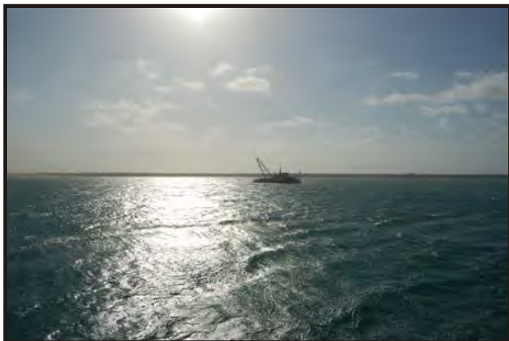
Figure 49: The barge, Ubejane , anchored on-site. A four-point spread is used over the wreck site. This allows the barge to be moved to any point on the wreck for lifting. (Photo V. Maitland)
