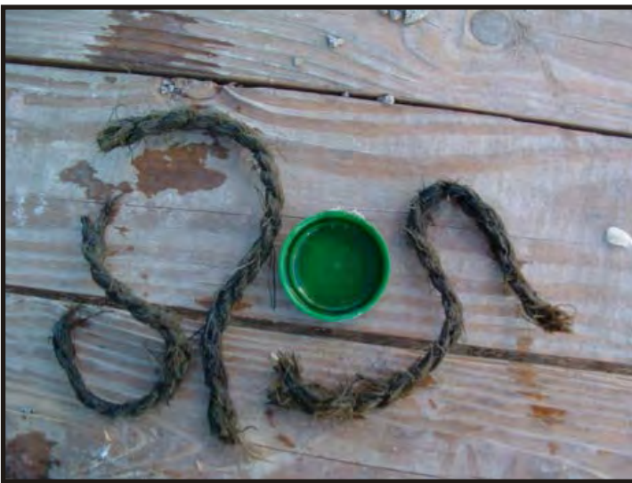
Figure 357: Lloyds' Survey of 1881 states that the ropes on the barque were manilla. These strands were made from two yarns. Normally strands were made by twisting three yarns together (Luce 1891:598). (Photo V. Maitland)
