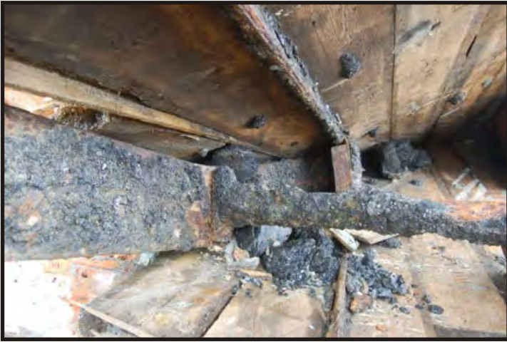
Figure 184: Heel attached to rider plate of the centre keelson. (Photo V. Maitland)
