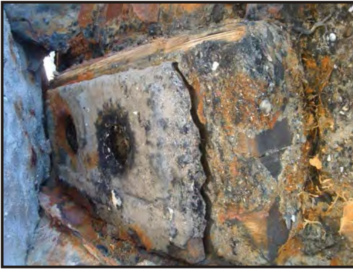
Figure 255: Close-up of hawseholes. Unlike the previous hawsehole,s the upper side is a solid cast slab with two pipes. There is a separating plank of wood between the bow plates and the upper end of the hawse pipe. (Photo V. Maitland)
