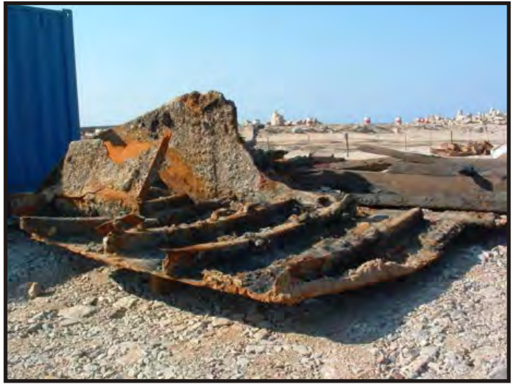
Figure 256: Section of side plating showing the rider plates where the vessel starts to narrow towards the bow. (Photo V. Maitland)
