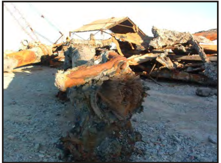
Figure 452: Close-up of the cap of the lower iron mast and the trunnion hoop around the wood. It appears there are shaped wooden wedges between the hoop and the wood top mast. The metal apparatus may have been to tighten the trunnion hoop. (Photo V. Maitland)
