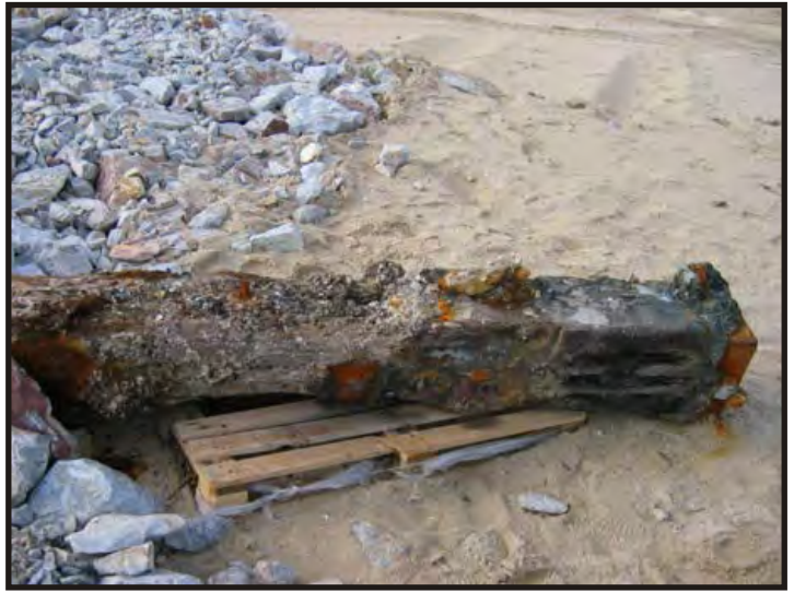
Figure 344: View from the top of the cathead, sheaves are visible on the right. (Photo V. Maitland)
