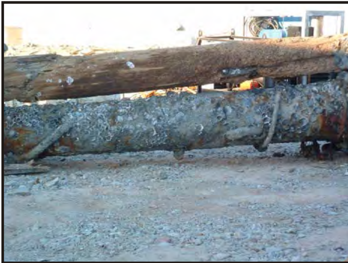
Figure 451: Close-up of the doubling. Cables from the rigging are still wrapped around the iron mast. (Photo V. Maitland)
