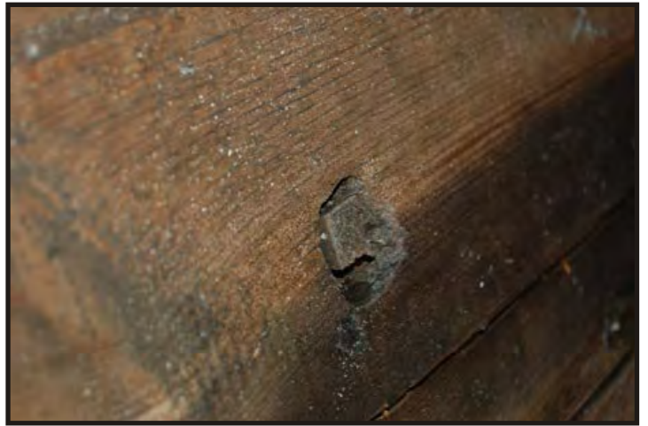
Figure 303: Wooden dowels are used intermittently throughout the cargo ceiling. I don't think these formed part of the attachment system as they were not carefully fitted or glued like the deck dowels. They may have been used as fillers for knot holes or other holes in the planks. (Photo V. Maitland)
