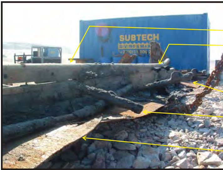
Figure 228: The channel projects from the sides of the ship and is used to give a greater spread to the lower rigging and backstays; this changed in later vessels to chain plate (Underhill 1938:108). In the County of Pembroke , the channel was on the inside of the bulwark. View of the channel from below, stanchions are visible, as well as the bottom of a dead-eye. On the far right of the channel are two metal projections, these go straight through the wood. There were various bits throughout sailing vessels for tying down rigging. (Photo V. Maitland)
