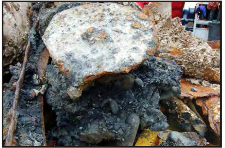
Figure 331: Top view of a possible gypsy. This piece of equipment was heavily encrusted with marine growth, it may be a different type of gypsy, perhaps for a larger windlass. (Photo V. Maitland)
