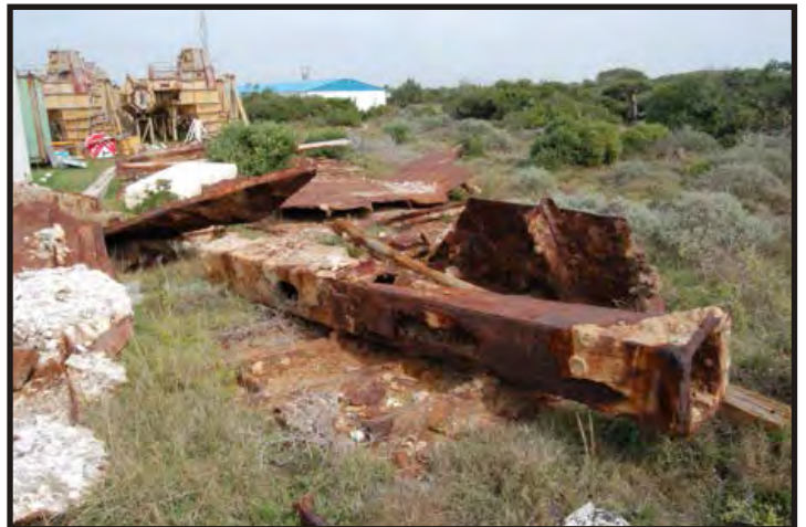
Figure 151: This square beam was recovered in 2004. It had two round holes in the side and is flanged on the end. (Photo V. Maitland)
