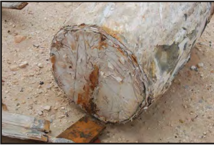
Figure 578: View of a cement barrel without the head. These barrels were lined with paper, possibly to absorb excess water during transportation. This was a precursor to the barrels being replaced by paper bags later in the 1900s. (Photo V. Maitland)
