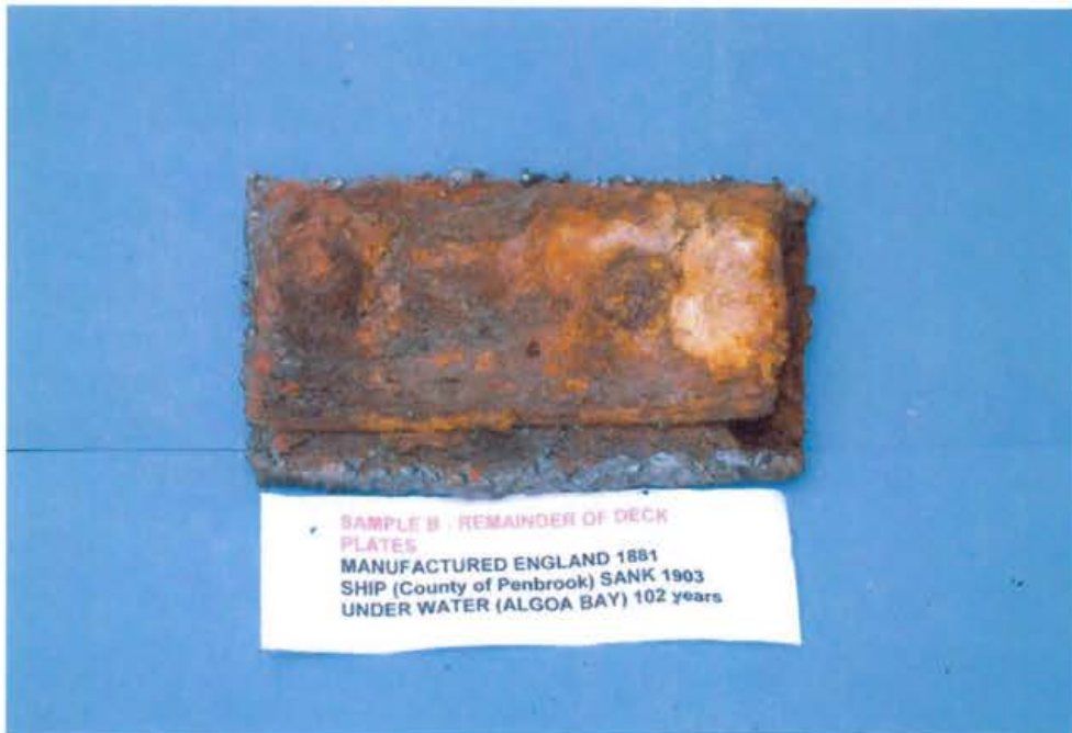
Figure 2: Photograph showing Sample B in the as-received condition.
