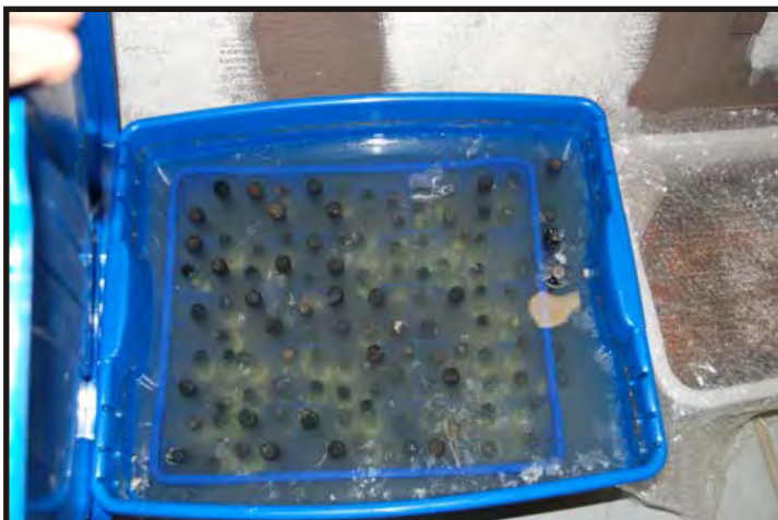
Figure 516: Unsealed castor oil bottles that were placed by Bayworld Museum in a saline solution. The leaking contents started to form hydrochloric acid. (Photo v. Maitland)
