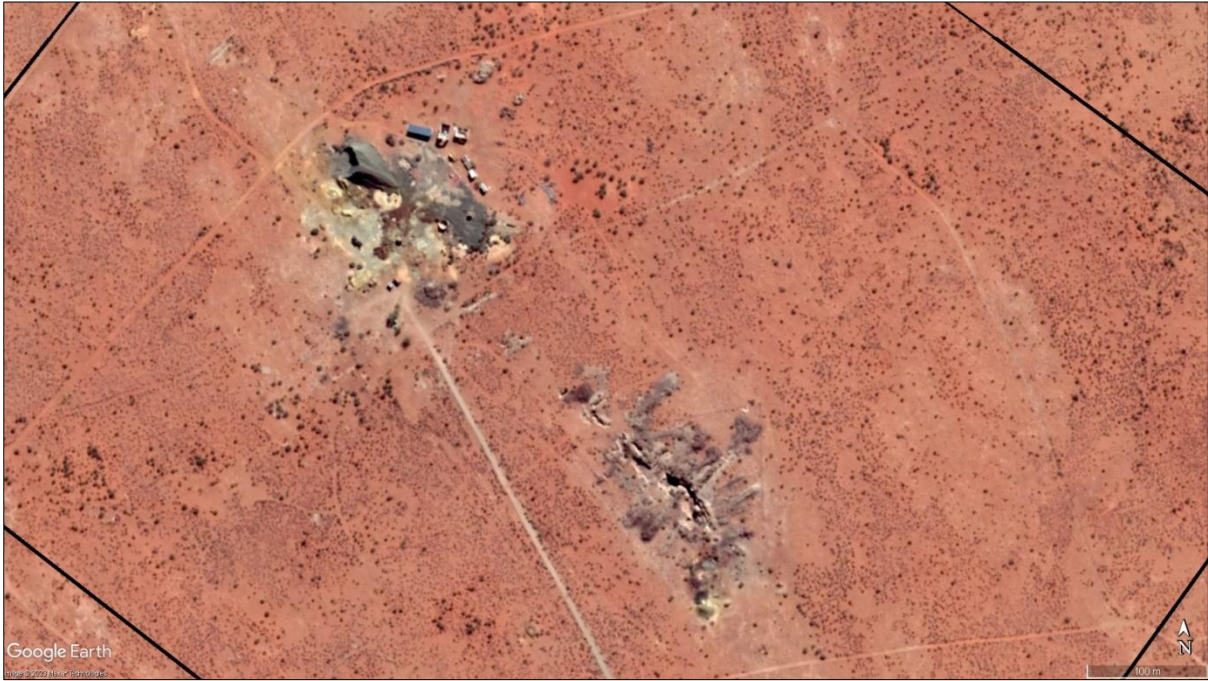
Figure 7: Detail of survey footprint indicating the mined areas (shaft and dumps (top) and opencast trenches (bottom)) (Google Earth Pro: 2023)
